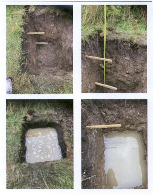
Existing ground water and rock not recorded at 1.0m BCL Infiltration test photographs
