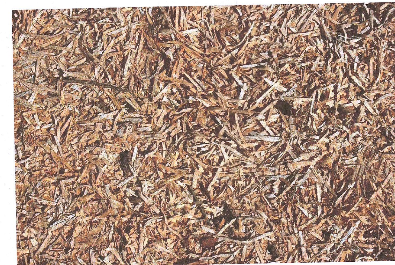
ENGINEERED WOOD CHIP SAFETY SURFACE - MIN. 200MM DEPTH. NOTE: CONFORMS TO EN 1177 EUROPEAN STANDARDS FOR PLAYGROUND SURFACING
