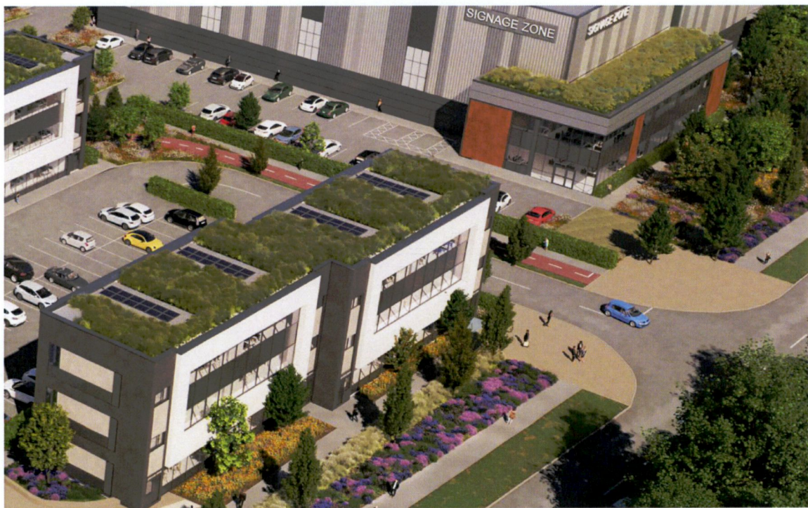
Extract from Aerial CGI View by others showing office units on Ballymount Avenue, with intensive green (brown) roofs to the office buildings. As described here, sufficient soil depth is proposed to allow for biodiverse planting on the roofs. (Please note this is an Artists' Impression; planting proposals are not accurate as per the species proposed, but show an overall impression in spatial and visual terms)
