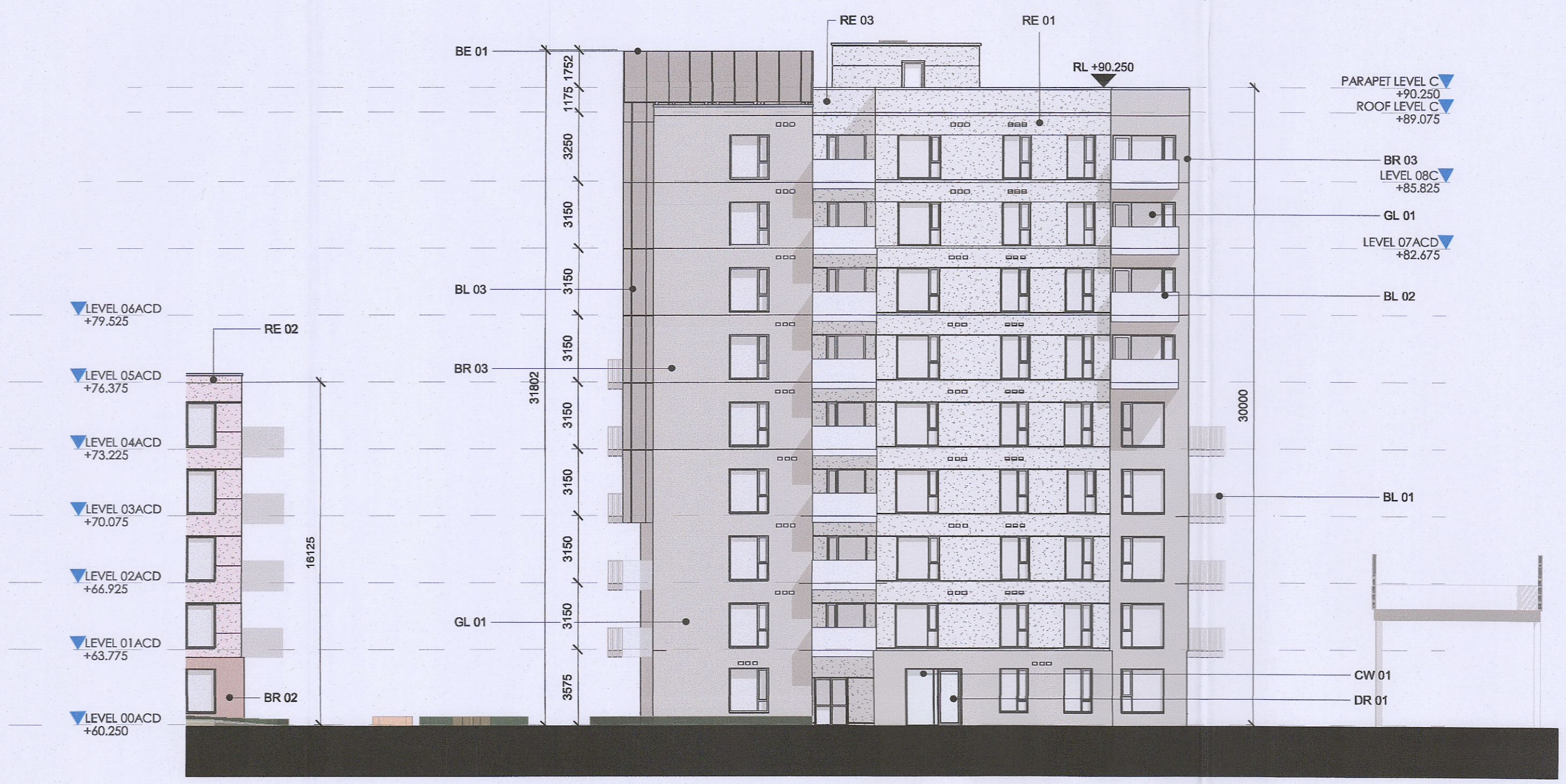
4 Block C - North Elevation 1 : 200
