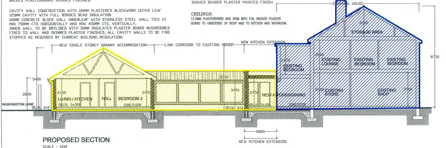
GROUND FLOOR TO BE 75MM THICK SCREED ON 100MM HIGH DENSITY KINGSPAN UNDER FLOOR INSULATION ON RADON BARRIER ON 200MM CONCRETE RAFT FOUNDATION ON 150MM WELL CONSOLIDATED HARDCORE.
