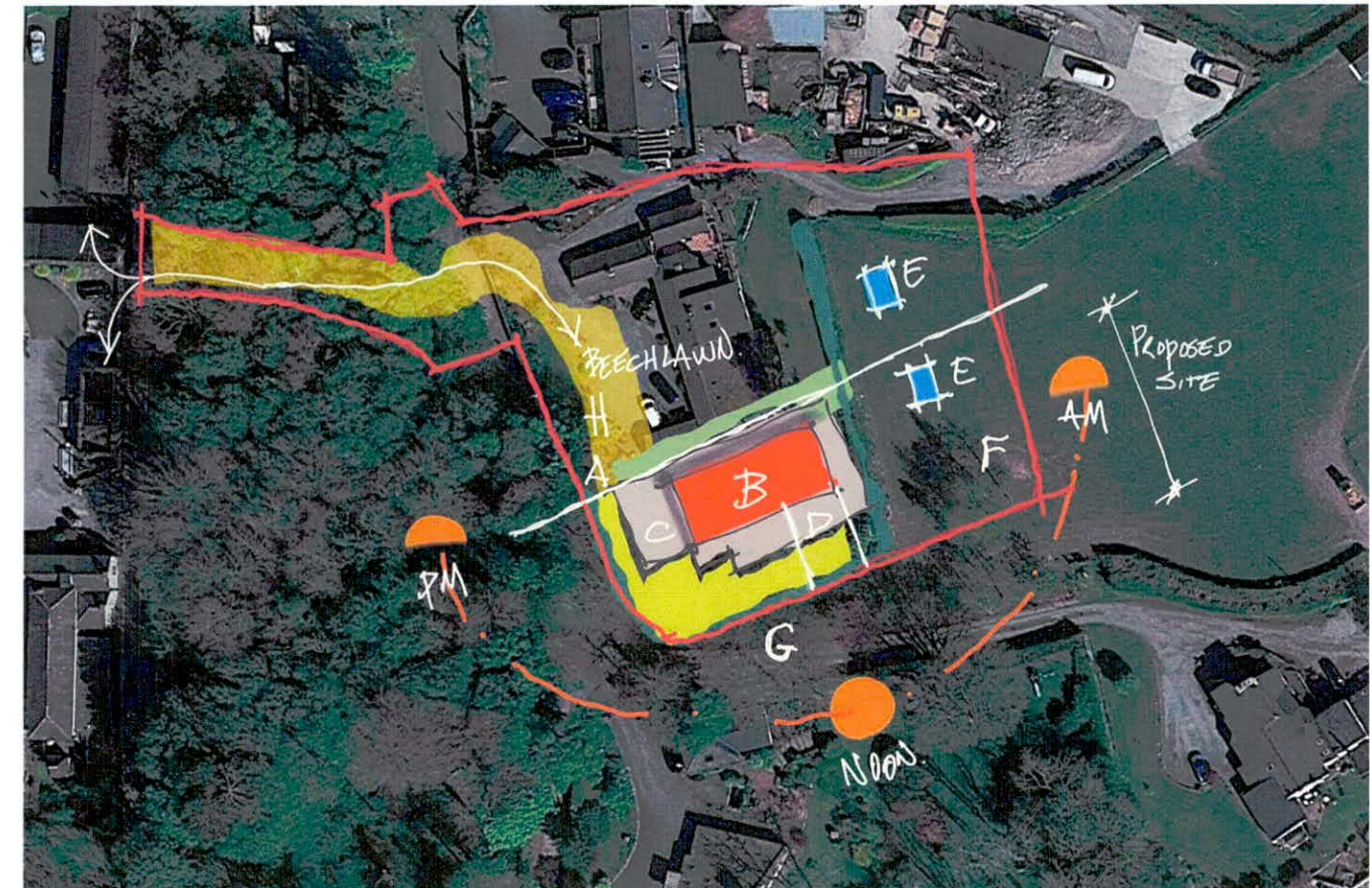
A – New boundary between properties. B – New house location. C – Parking & Bins. D – Tiered gardens. E – New Biocycles. F – Views downhill east toward coast. G – Proposed well. H – Proposed Access.
