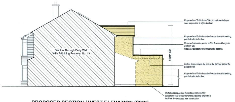
PROPOSED SECTION / WEST ELEVATION (SIDE)
