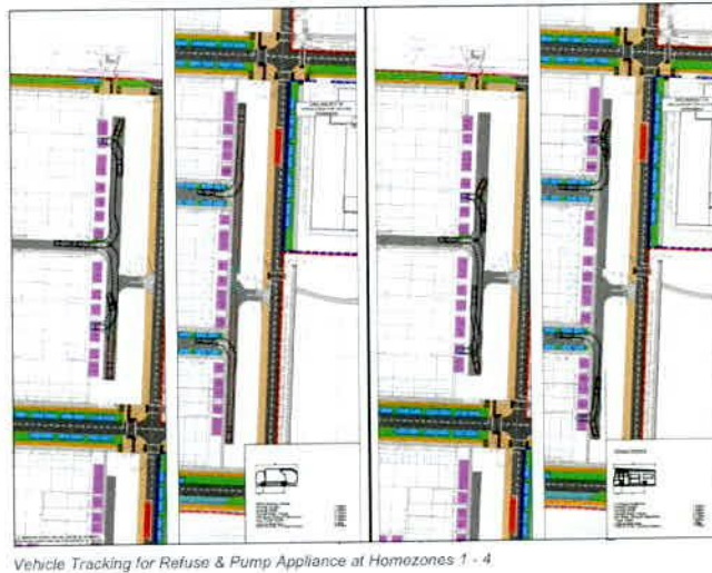
Figure 1: Extract from Memo, prepared by Atkins Consulting Engineers showing Refuse Vehicle and Pump Vehicle Tracking for the 4no. proposed Homezones.
