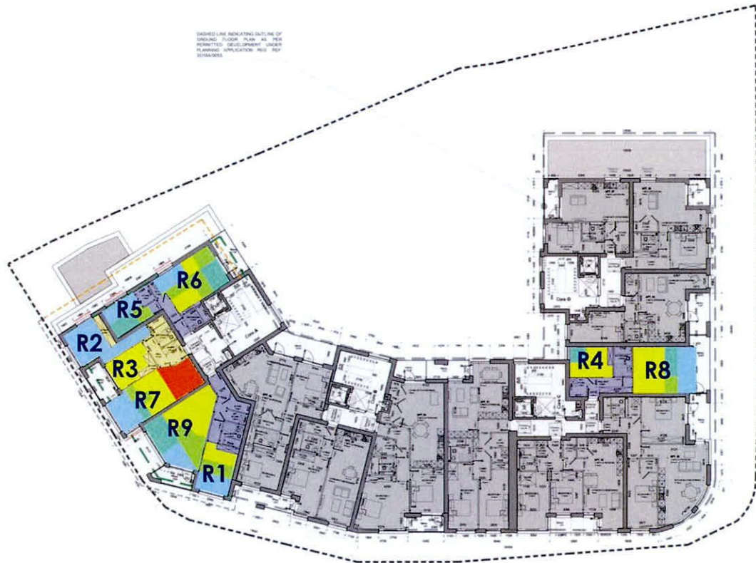
Reference Image 17: Second Floor – Daylight Factor Analysis
