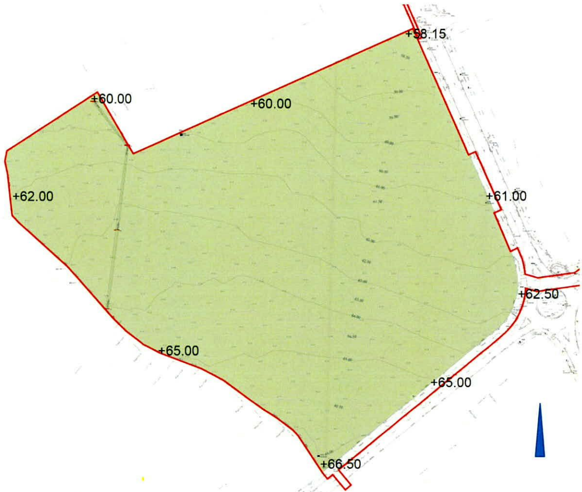
Site Survey and Analysis Plan, showing the grassed surface, devoid of trees, hedges or other landscape features; Topography: Site is almost flat with average gradient of 1:40 (2.5%)
