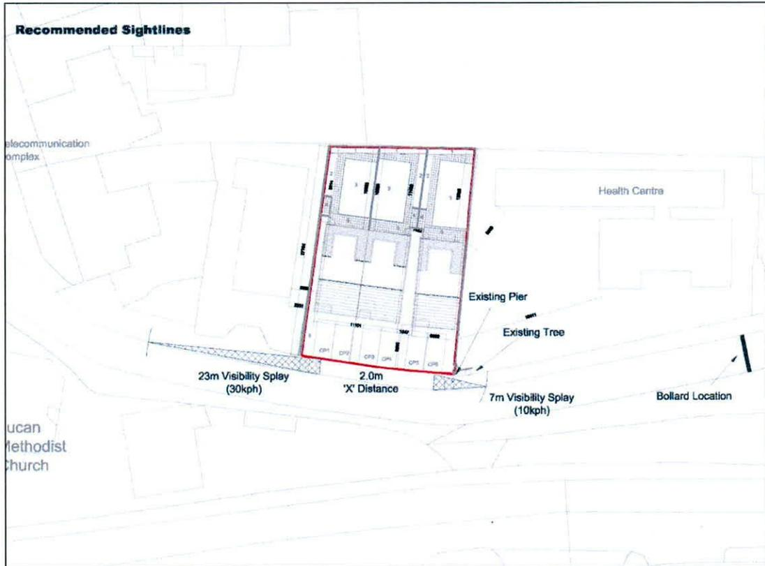
**Figure 1.6: Recommended Sightlines to Right and Left of Car Parking Spaces (Source of Background Mapping: PAMES)**
