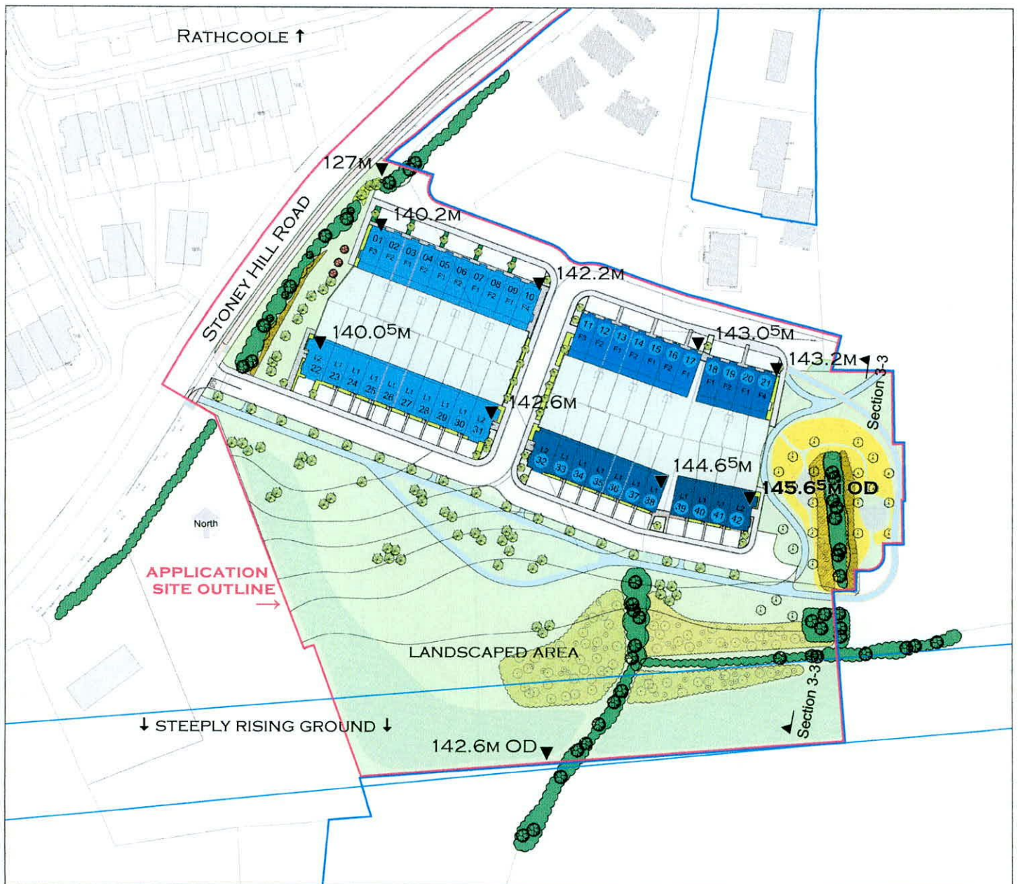
SITE PLAN OF PROPOSED DEVELOPMENT WITH ELEVATIONS (O.D.) OF HIGHEST PARTS SCALE 1:1500 APPROX.
