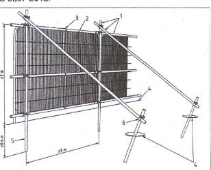
Heavy gauge 2 m tall galvanized tube and welded mesh infill panels Panels secured to uprights and cross-members with wire ties
