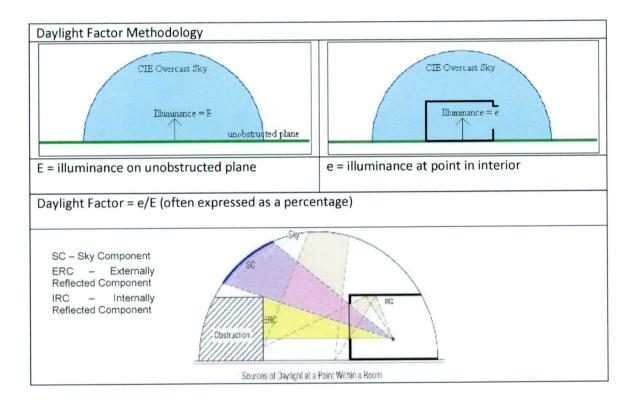
Both illuminances are measured under the same standard sky, a CIE overcast sky. Since the sun is in a particular position for only a short period each day, direct sunlight is excluded. Instead diffuse sunlight is used for average daylight calculations. Diffuse sunlight describes the sunlight that has been scattered by molecules and particles in the atmosphere but has still made it down to surface of the earth.
