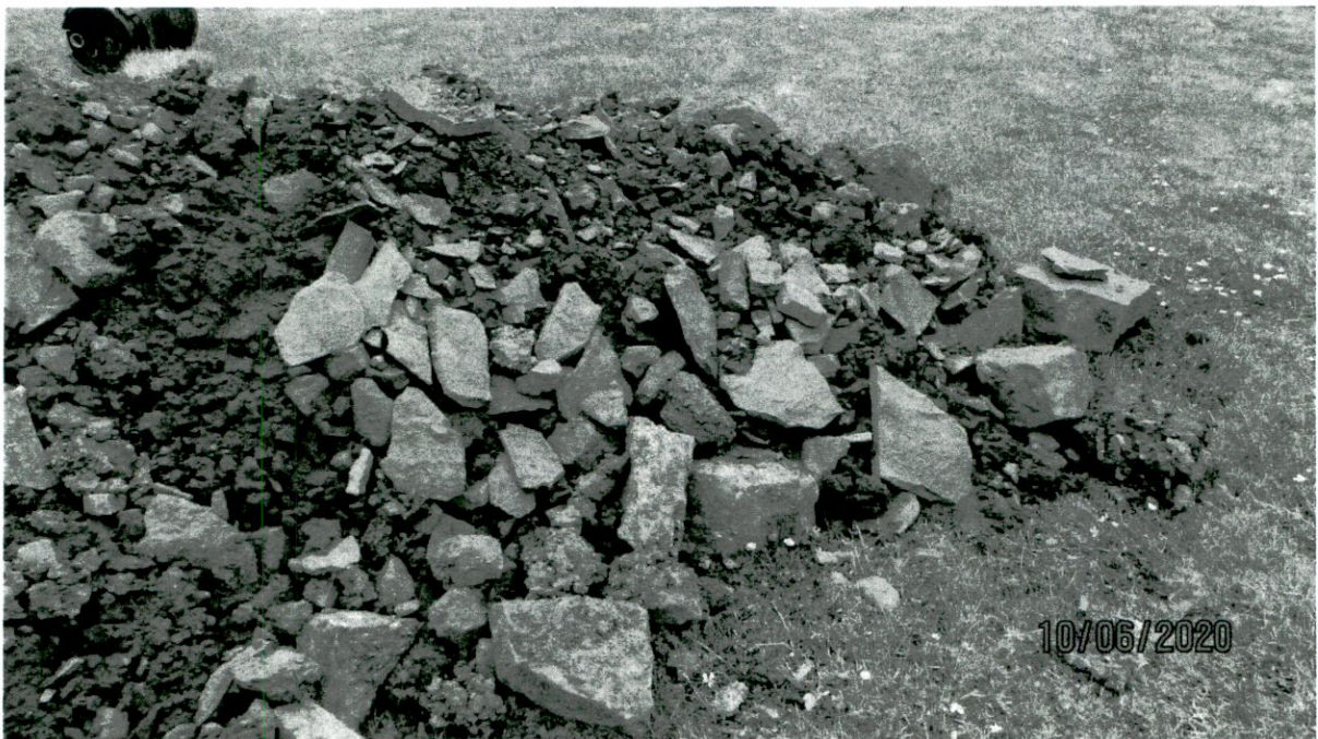
Photo No 14: Rock. Rock encountered at 2.3M deep. Could not dig through. Bedrock.
