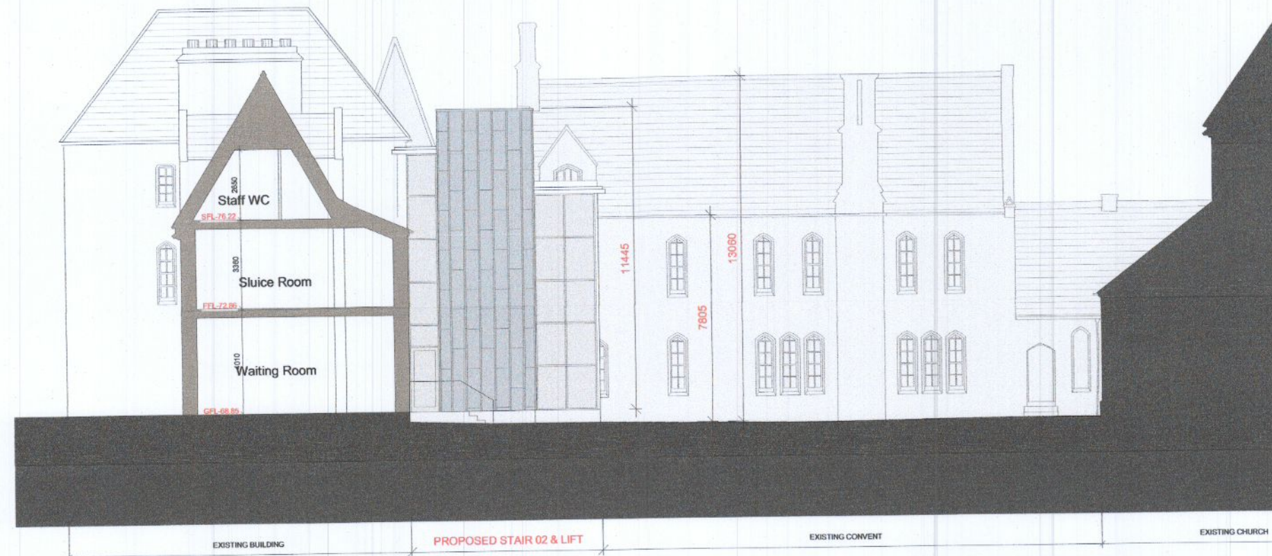
Elevation-07 - East Elevation - Courtyard - Scale 1:200
