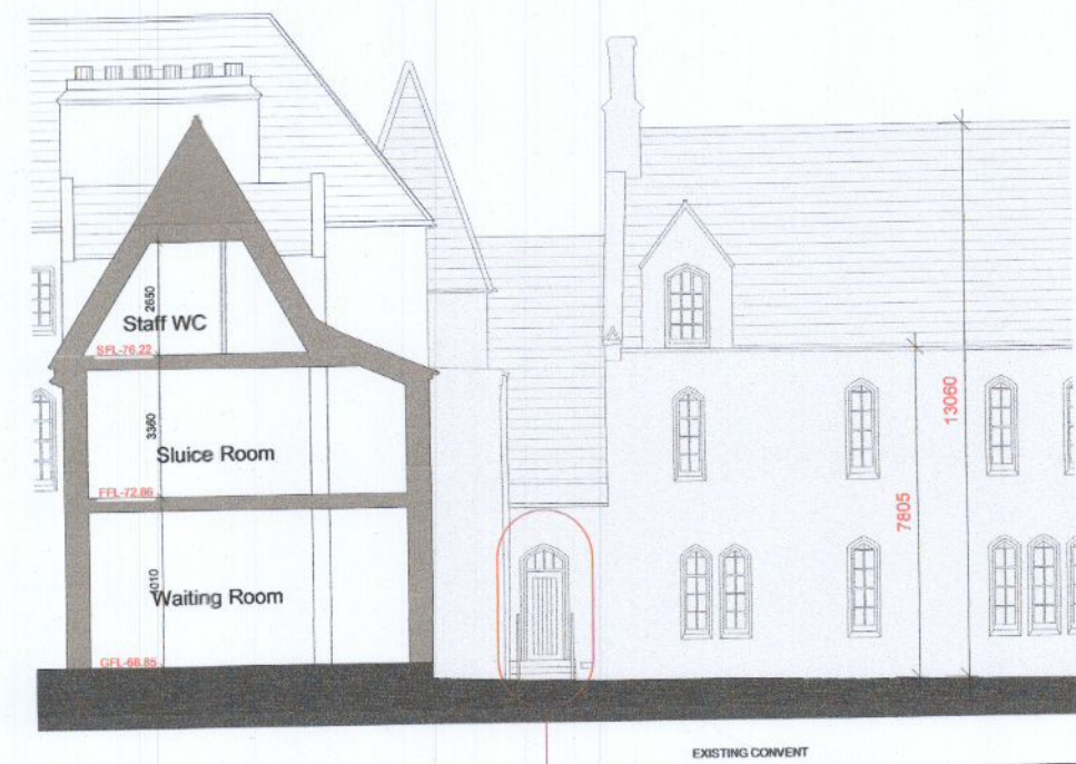
Elevation-07 - Part East Elevation - Courtyard - Scale 1:200
