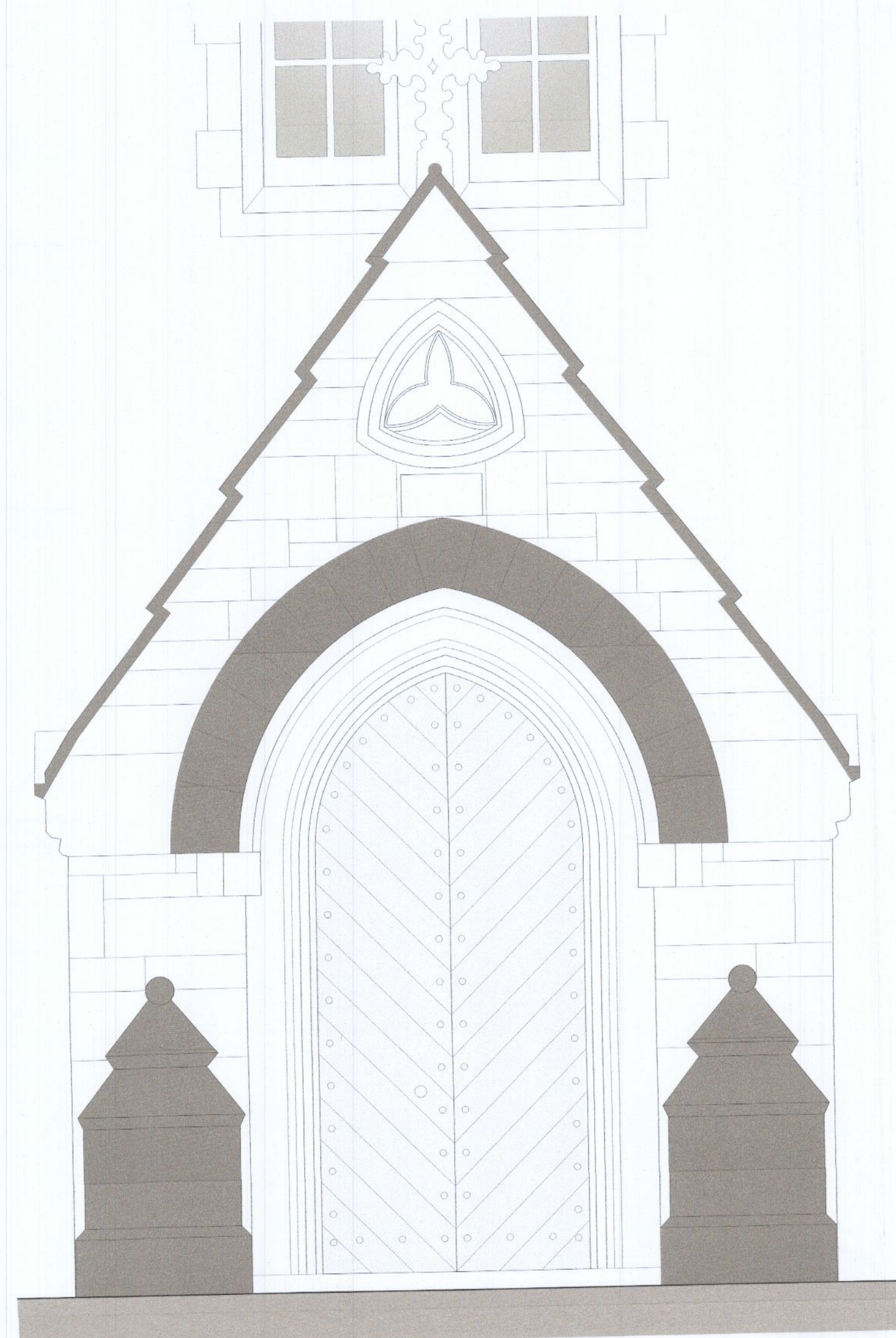
EXISTING ENTRANCE (EAST ELEVATION) Existing Door Which Currently Opens Inwards to be Modified to Open Outwards
