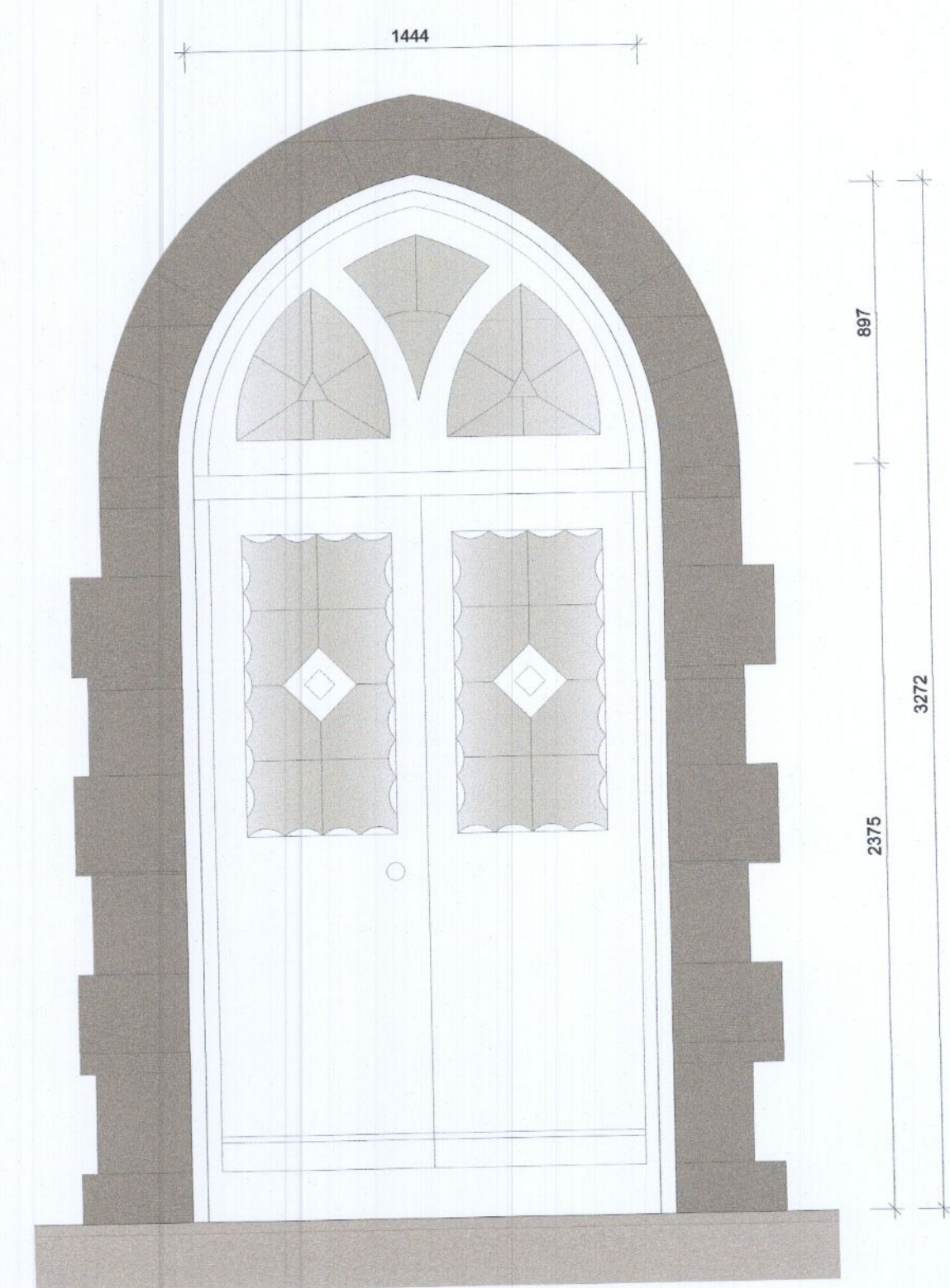
EXISTING DOOR WITH STONE SURROUND (COURTYARD WEST ELEVATION) Existing Door Which Currently Opens Inwards to be Modified to Open Outwards
