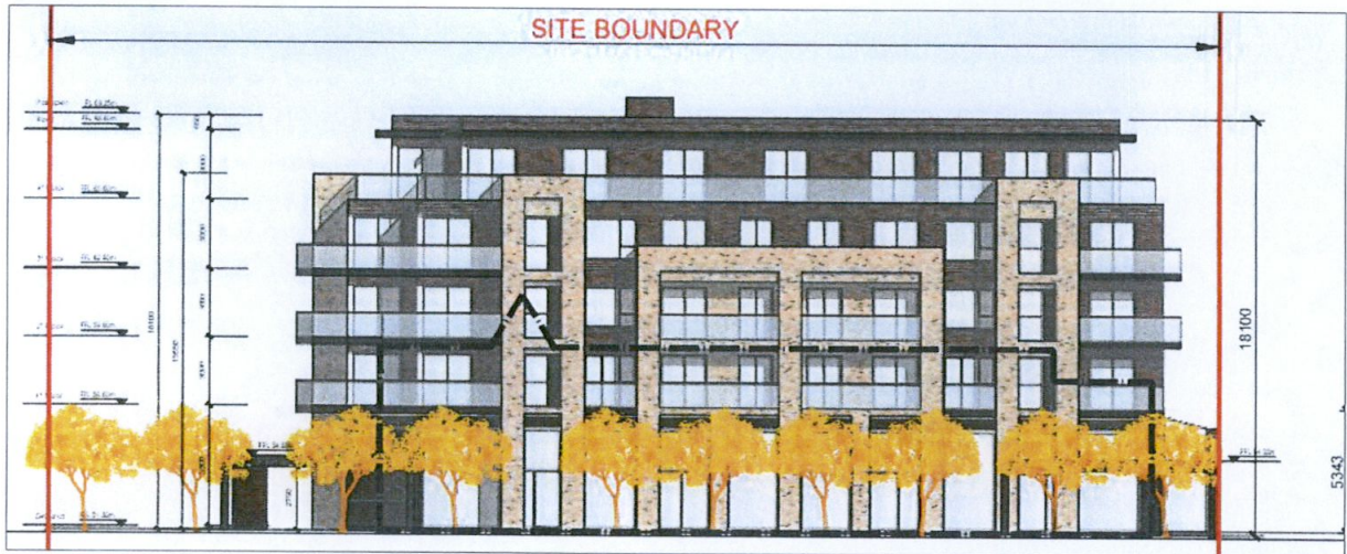
Figure 4: Proposed elevation, modern urban features, use of brick and vertical windows to reduce perceived massing
