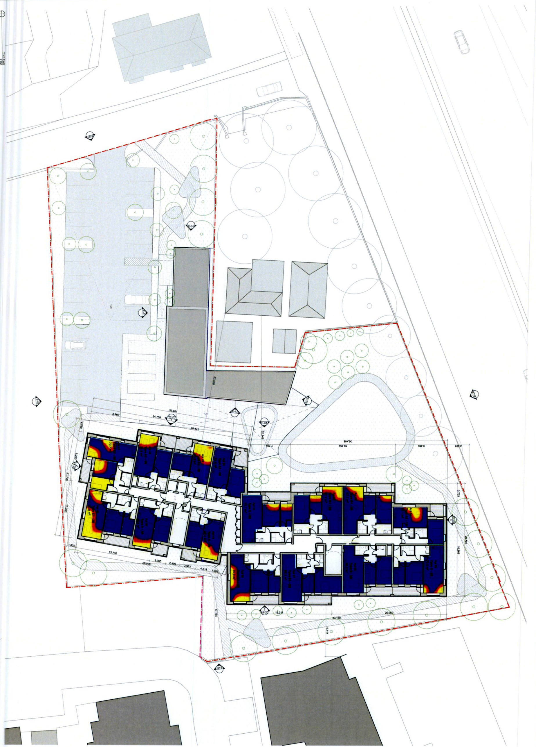
THIRD FLOOR PLAN - MINIMUM 3 HOURS OF SUN ACCESS PER DAY, 21st March
