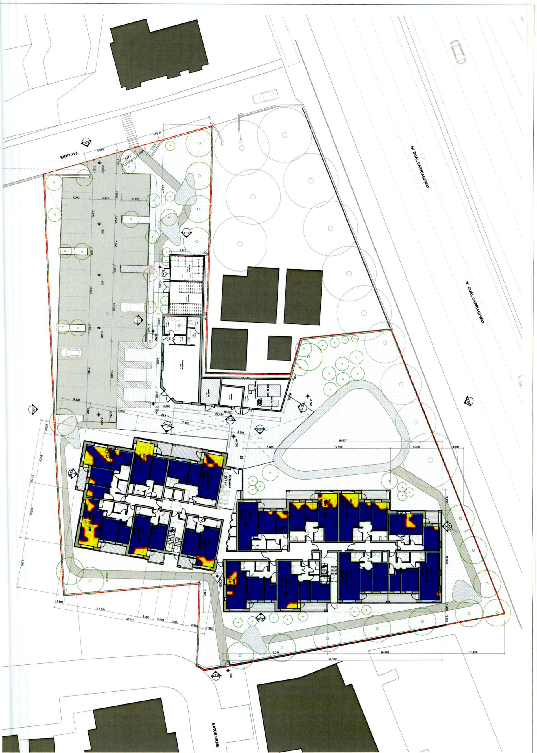
GROUND FLOOR PLAN - MINIMUM 3 HOURS OF SUN ACCESS PER DAY, 21st March
