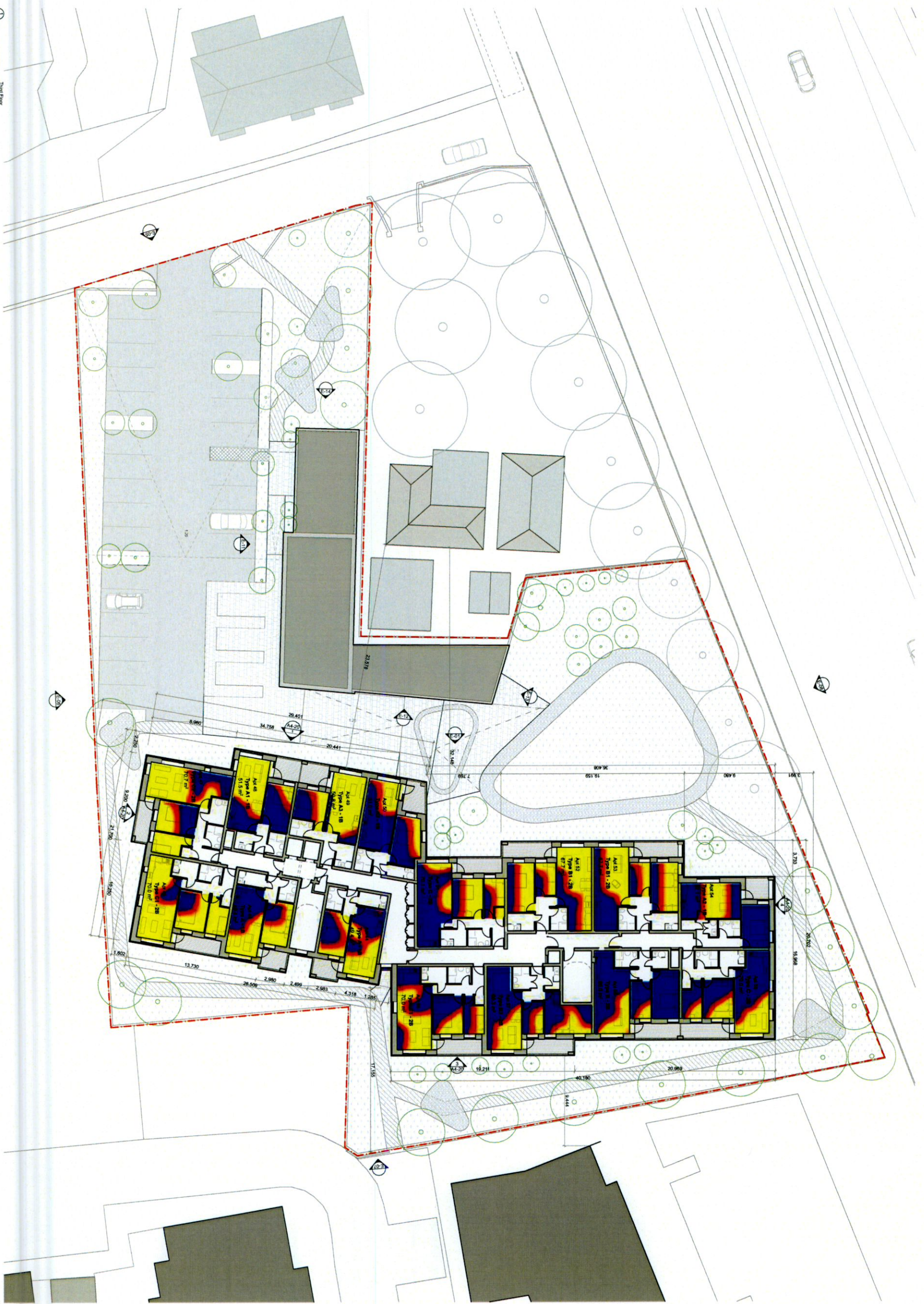
THIRD FLOOR PLAN - MINIMUM 1 HOUR OF SUN ACCESS PER DAY, 21st March
