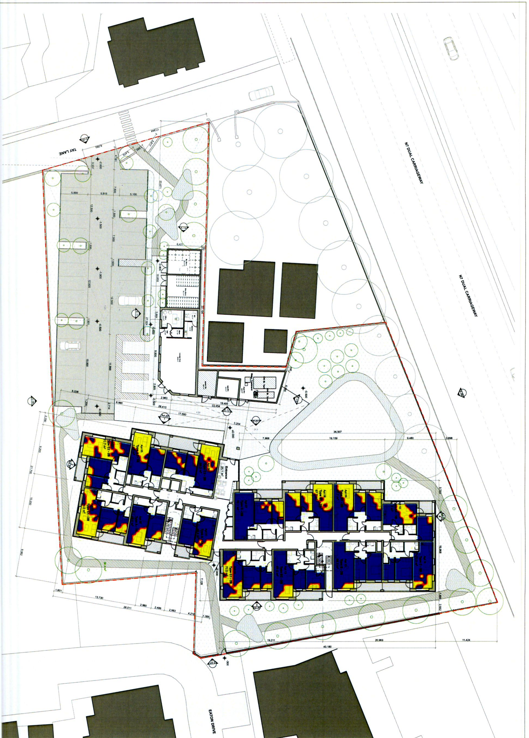
GROUND FLOOR PLAN - MINIMUM 2 HOURS OF SUN ACCESS PER DAY, 21st March
