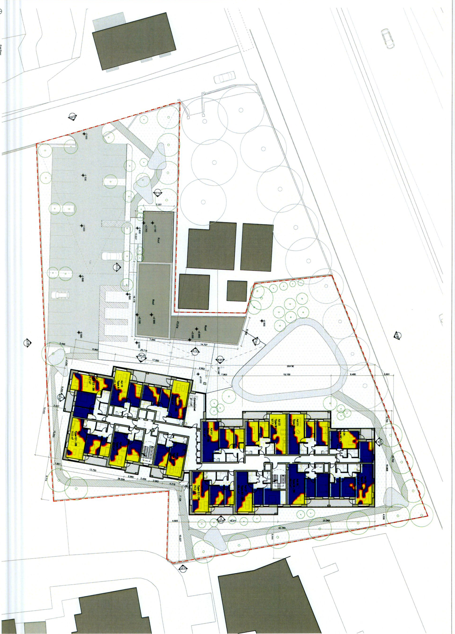
FIRST FLOOR PLAN - MINIMUM 1 HOUR OF SUN ACCESS PER DAY, 21st March
