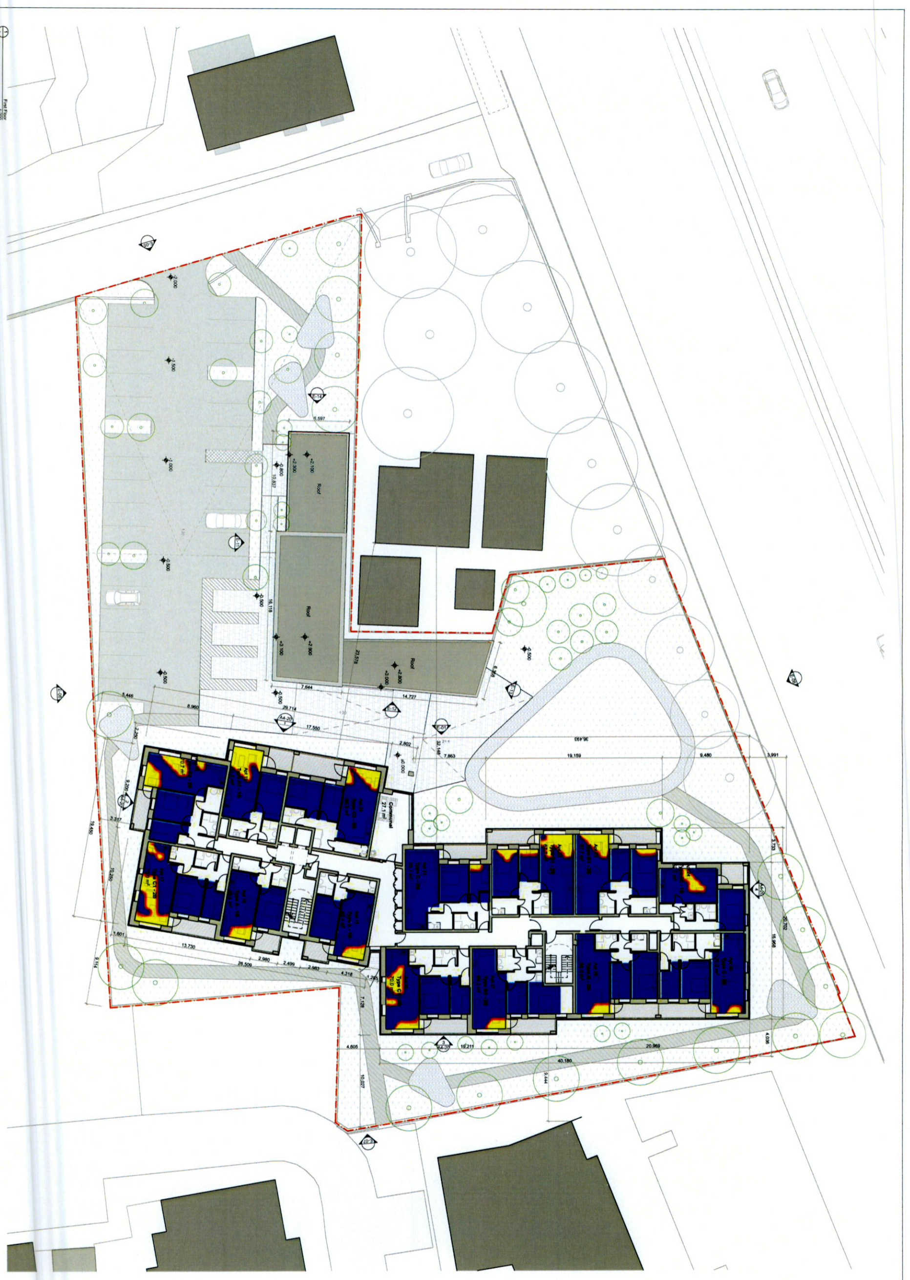
NOTES: FIRST FLOOR PLAN - MINIMUM 3 HOURS OF SUN ACCESS PER DAY, 21st March
