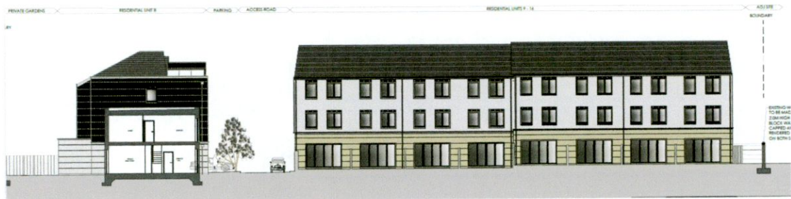
Figure 2 – Contiguous section-elevation - Site Section 4-4 which is taken through the rear gardens of units 9 to 16 and through unit 8, facing Tara Crescent & the Green. Note three storey impact with slated roof.
