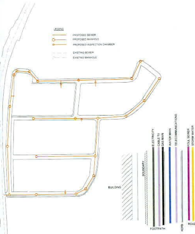
TYPICAL LAYOUT FOR SEWER WITHIN NEW DEVELOPMENTS DRAWING No. STD-WW-02
