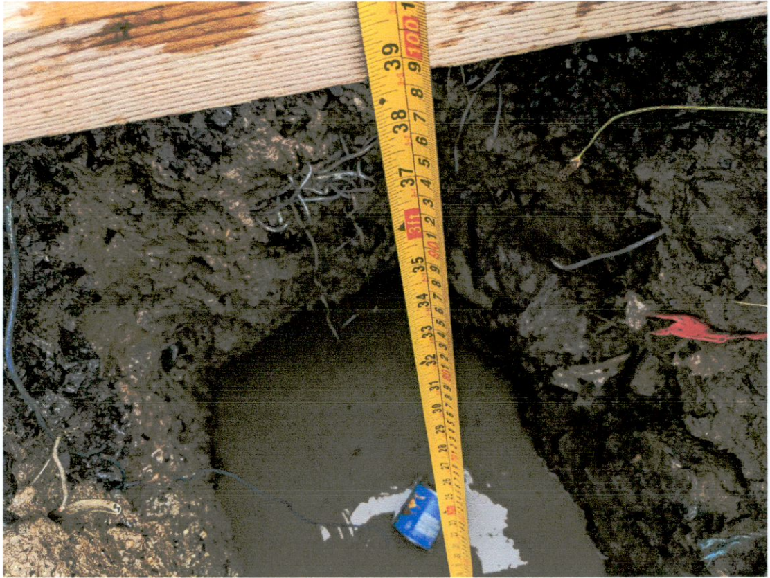
#05 – Immediately after 3 rd fill, 29 th July 2022, Top of Water to Ground Level – 980mm.
