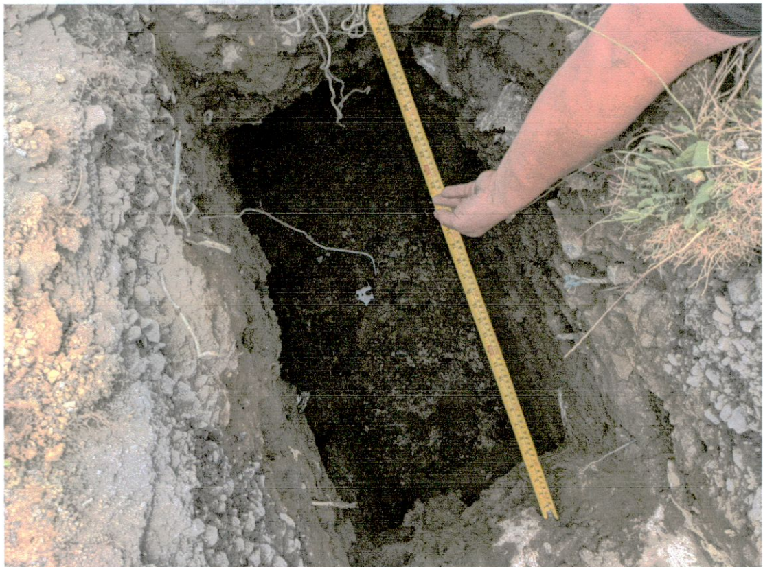
#02 – Trial pit before 1 st fill, 27th July 2022.
