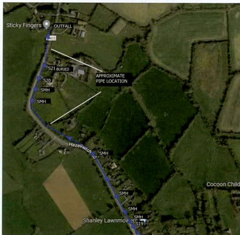
Figure 4.2: Northern extent of existing surface water network on Hazelhatch Road (Source: CCTV Report from Planning reference SHD3ABP-313814-22)
