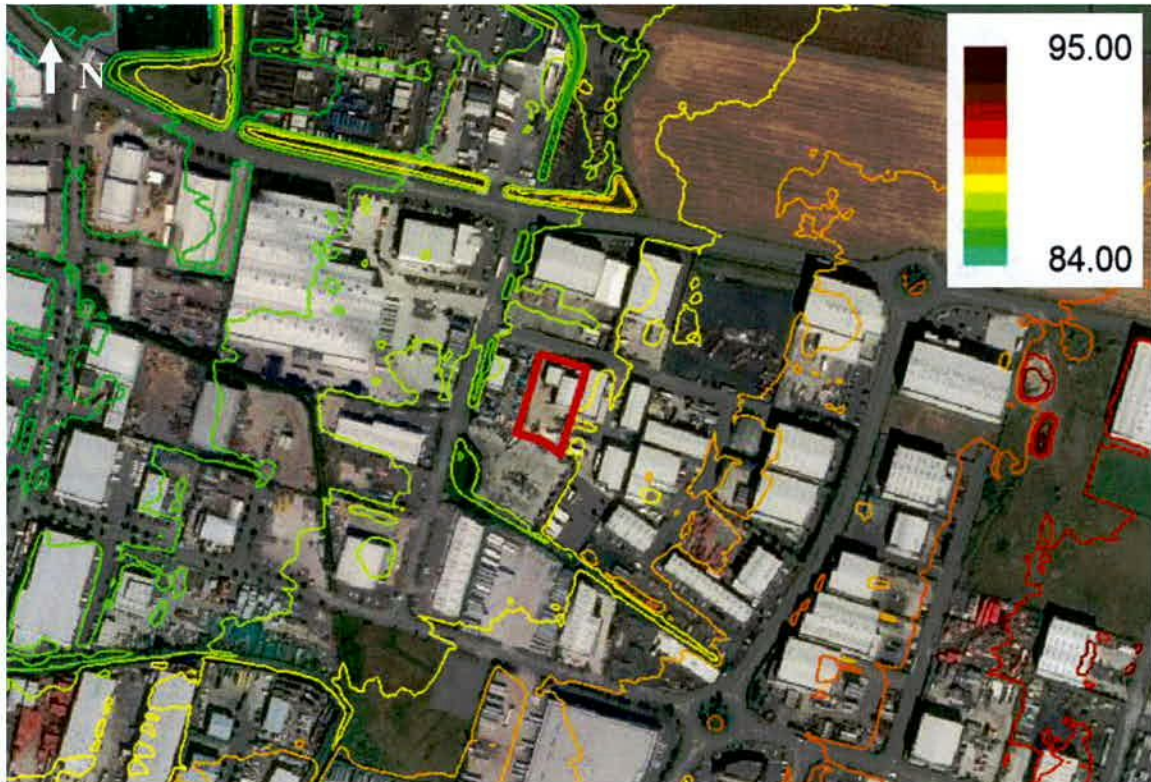
Figure 6.3: Topographic Data from LiDAR
