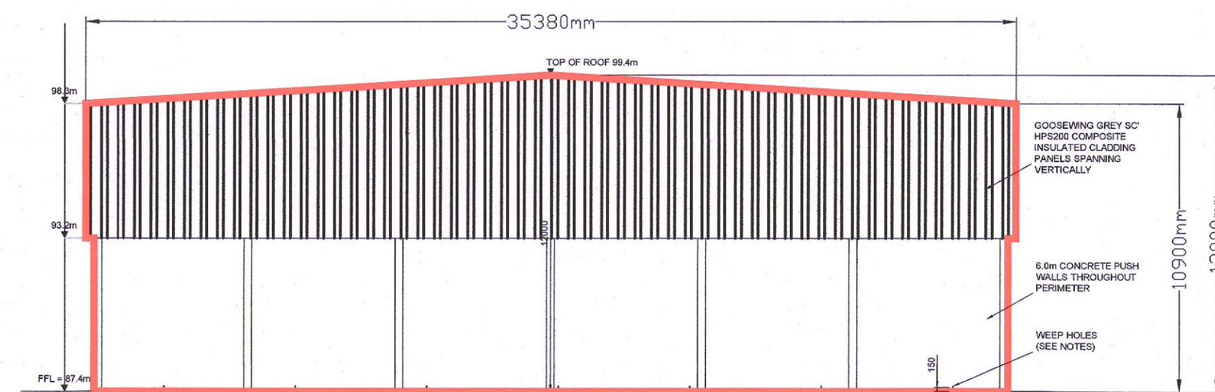
PROPOSED REAR ELEVATION (SOUTH) Scale 1:200
