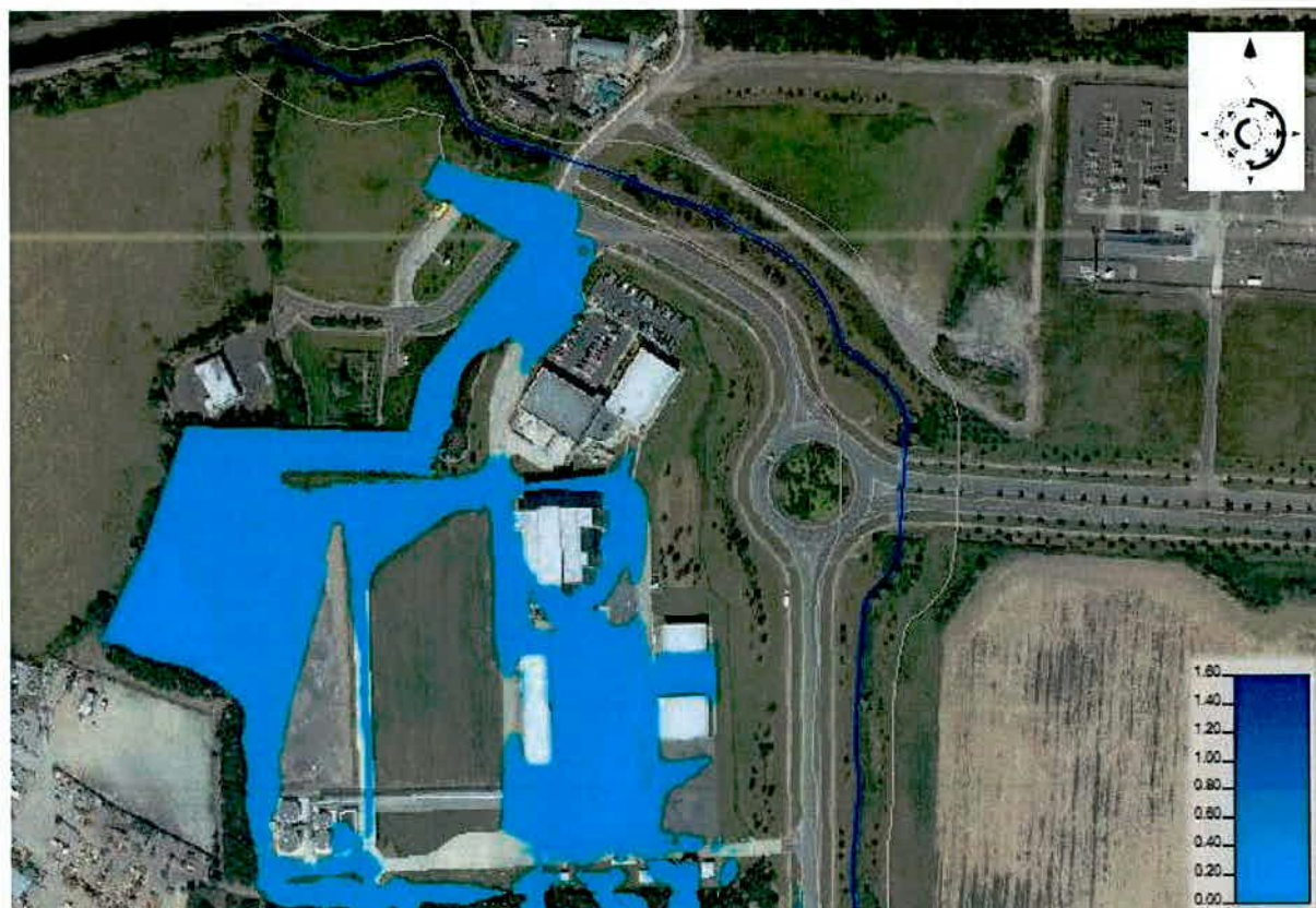
Figure 11 – Flood depth on existing Takeda site for 1% AEP MRFS event with new development
