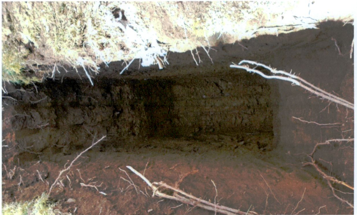
Trial Pit – Depth 2.4m
