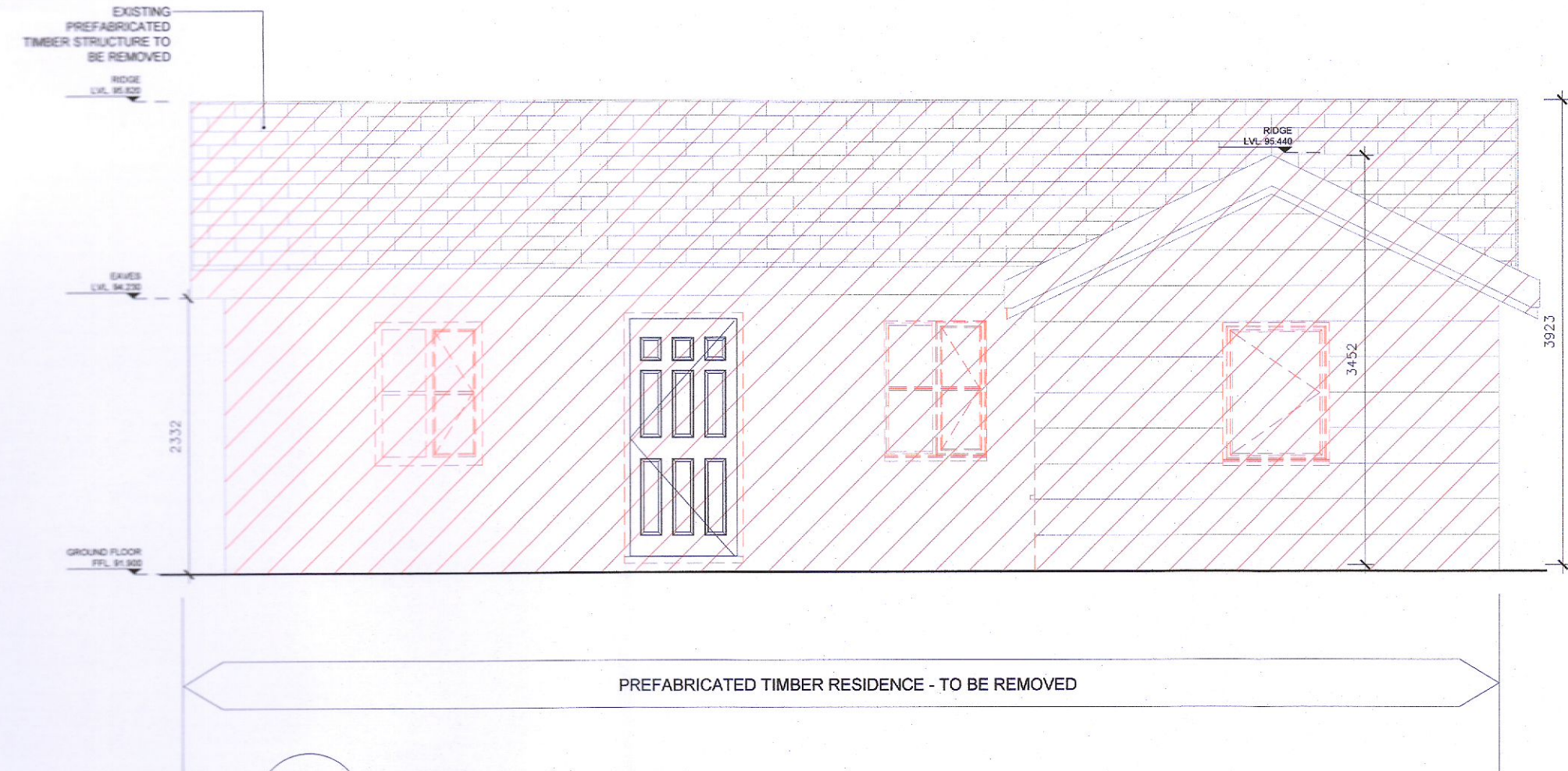
01 Building B - Existing North Elevation EX 302 1:50
