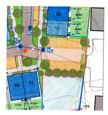
**Image 1:** This image donates the proposed connection point between the proposed development and the adjoining existing development (Market Square). This has been poorly designed as the connection point proposed does not line up with the existing provisions.
