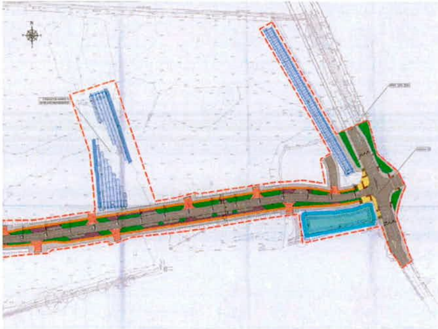
Fig. 16 – permitted surface water attenuation under Ref. SDZ20A/0021 on the subject application site.
