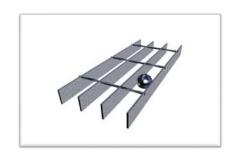
Safegrid / Flowforge general utility steel grating comprises of a series of parallel, flat, load bearing bars at equal spacing. These are held upright by 6mm twisted-square transverse bars that are resistance welded into the top surface. With no ball proof rating General Utility grating shall be used where there is no risk of personnel passing below.
