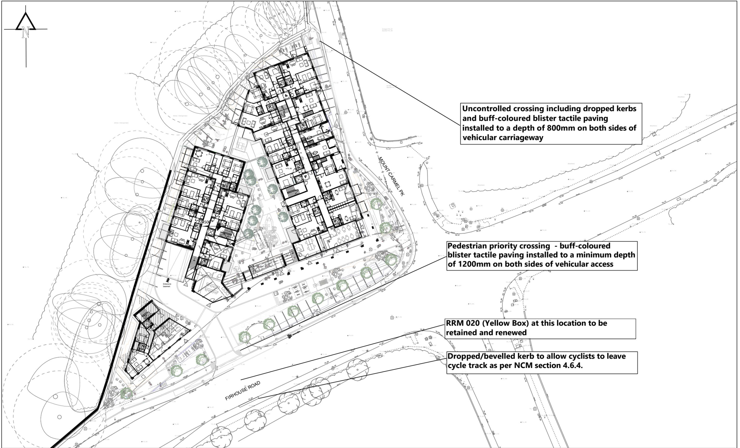
**Uncontrolled crossing including dropped kerbs and buff-coloured blister tactile paving installed to a depth of 800mm on both sides of vehicular carriageway**
