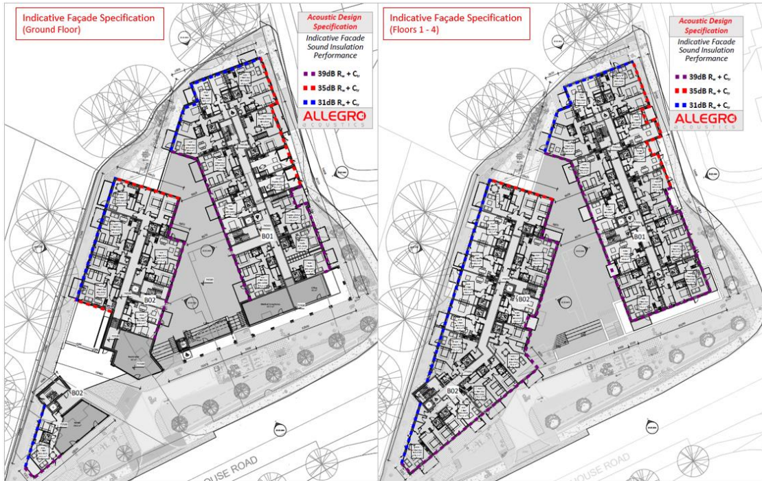
Figure 7: Indicative façade insulation sound insulation requirements.
