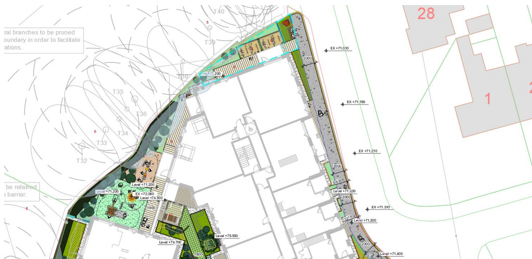
Figure 19. Landscape plan at LG level showing streetscape of 2.00m width footpath along Mount Carmel Park; location of mesh fencing and gate to secure creche site; location of creche staff cycle shelters; and of shallower attenuation tank under cycle shelters
