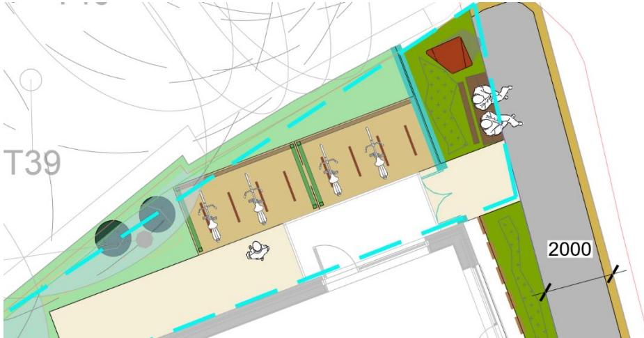
Figure 24. Detail of landscape plan illustrating location of cycle parking in green-roofed shelters for creche staff at northern corner of site
