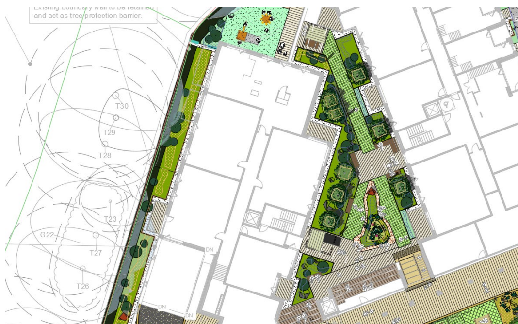
Figure 26. Landscape plan detail of communal amenity open space provided in the podium courtyard.
