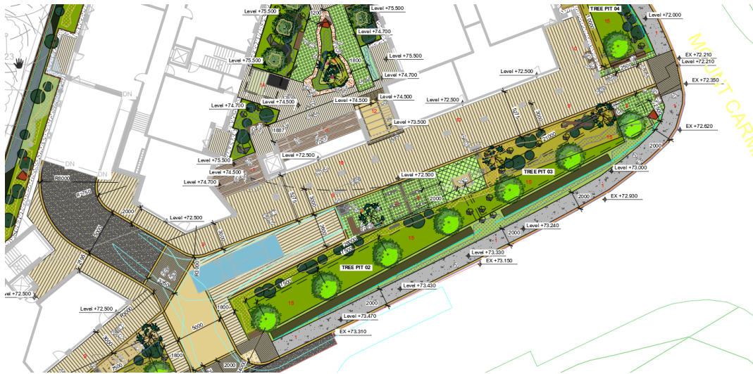
Figure 17. Detail of current landscape plan illustrating public open space to the south of the building, with wider 3.00m path, sheltered arcade under the building, increased play provision along the playful route and increased tree and amenity landscape planting
