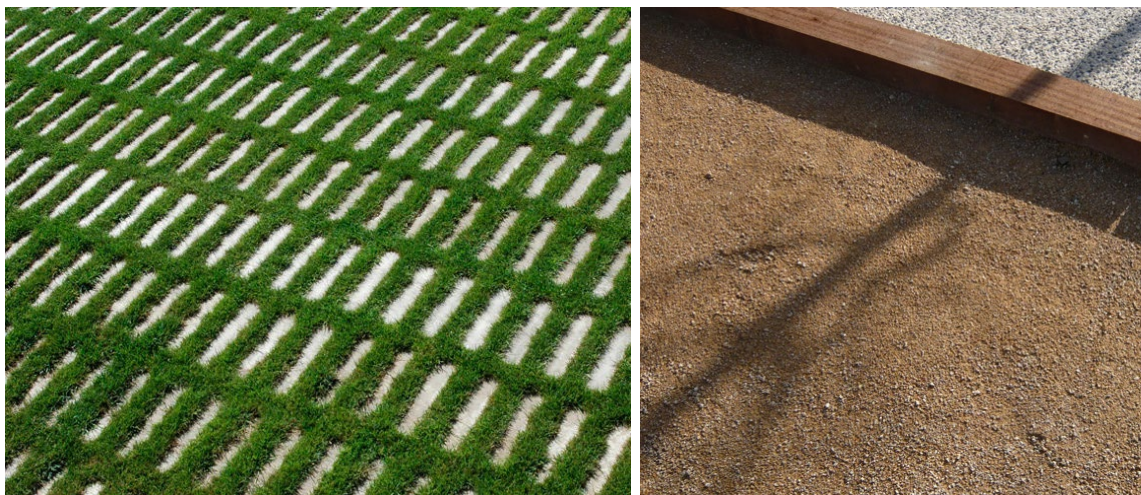
Figure 40. Permeable paving of grass-pave ('Redes' by Escofet) and golden coloured self-binding golden gravel
