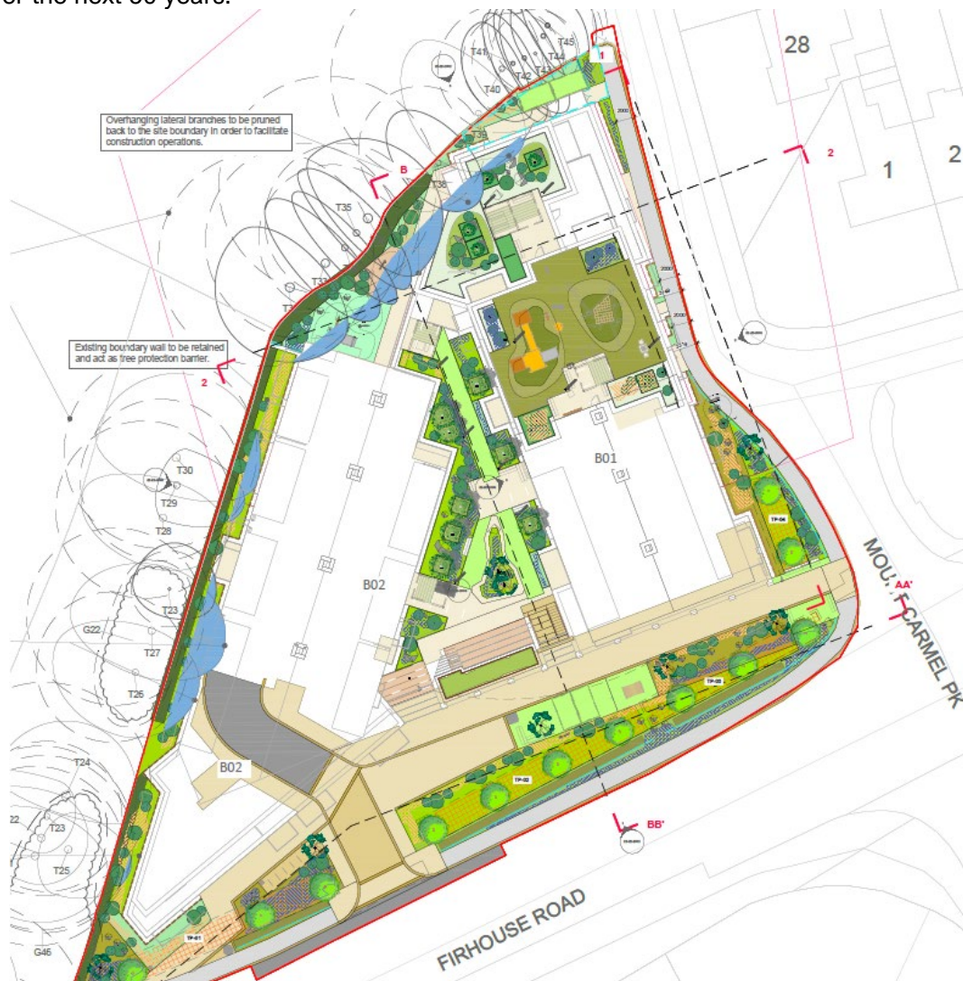
Figure 54. Landscape Plan with SuDS tree Pits illustrated with orange hatch in public open space
