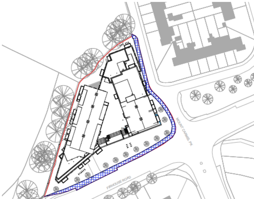
Figure 9. Detail of ‘Taken In Charge Plan’, prepared by OMP Architects, illustrating the area to be taken in charge by the local authority with a blue hatch
