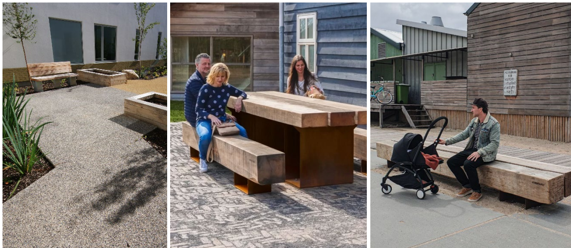
Figure 39. In situ concrete paving treated with an exposed aggregate retarder to 2.00m width path along the public road; durable picnic sets, benches and seats provided through the public and communal amenity open space
