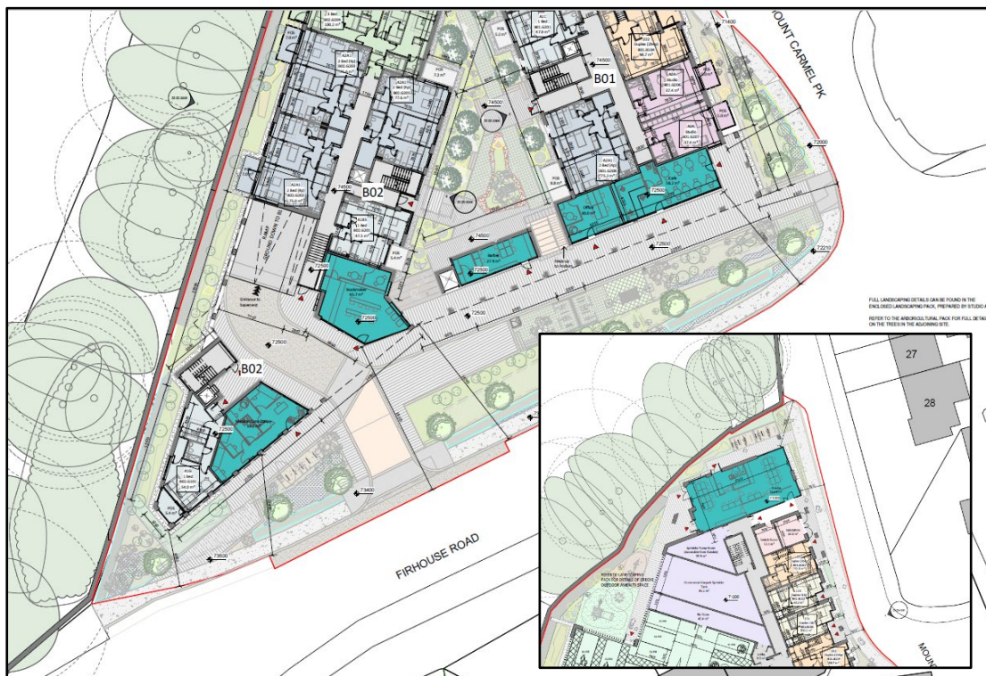
Figure 4.2: Extracts from the proposed Ground Floor Plan (Level 00) and Lower ground Floor Level (Level B1) plans, prepared by OMP Architects showing the proposed non-residential uses.
