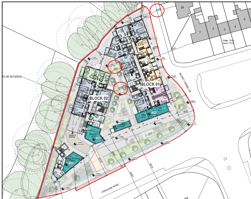
Figure 2.2: Extract from Dwg. no. 20022-OMP-00-SP-DR-A-1000 (Proposed Site Plan layout) showing the instances where the 22m separation distance is not met with measurements circled in red (source: OMP Architects.)
