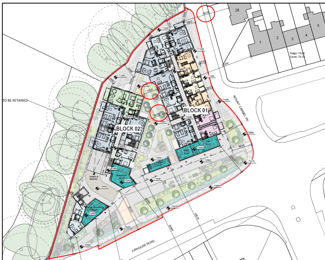
Figure 2.4: Extract from Dwg. no. 20022-OMP-00-SP-DR-A-1000 (Proposed Site Plan layout) showing the instances where the 22m separation distance is not met with measurements circled in red (source: OMP Architects.)
