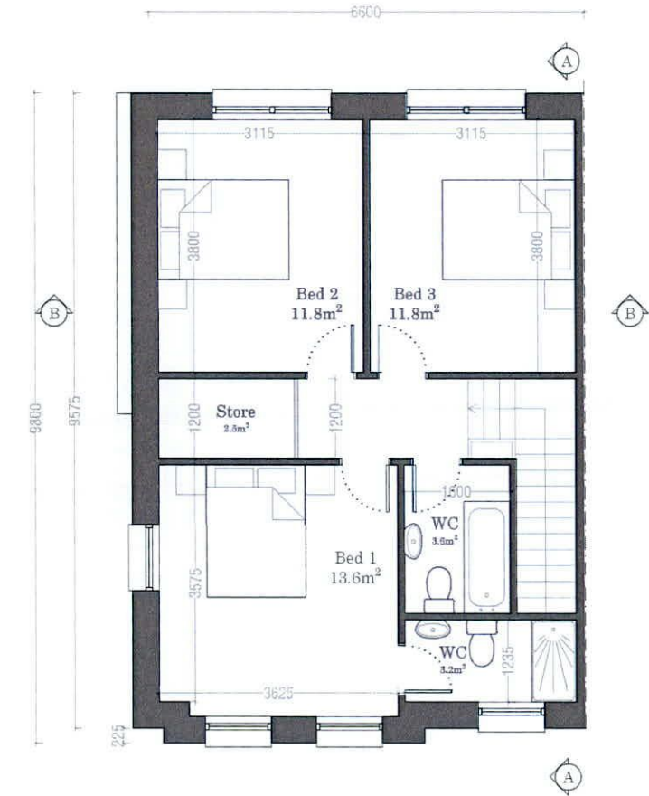
House Type A2 - End Terrace First Floor Plan 56.2m 2
