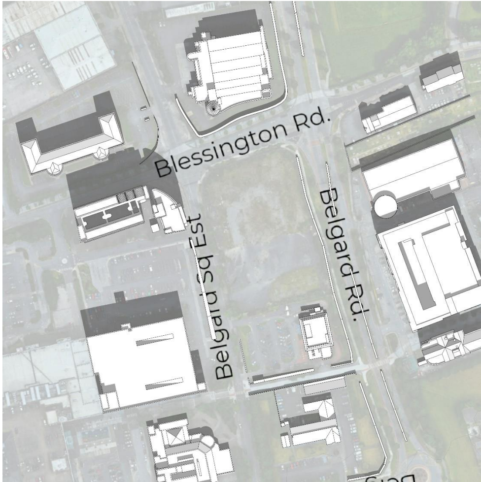
Shadows Cast at 12pm (UTC+0) on the 21 st March - Before Development Scenario
