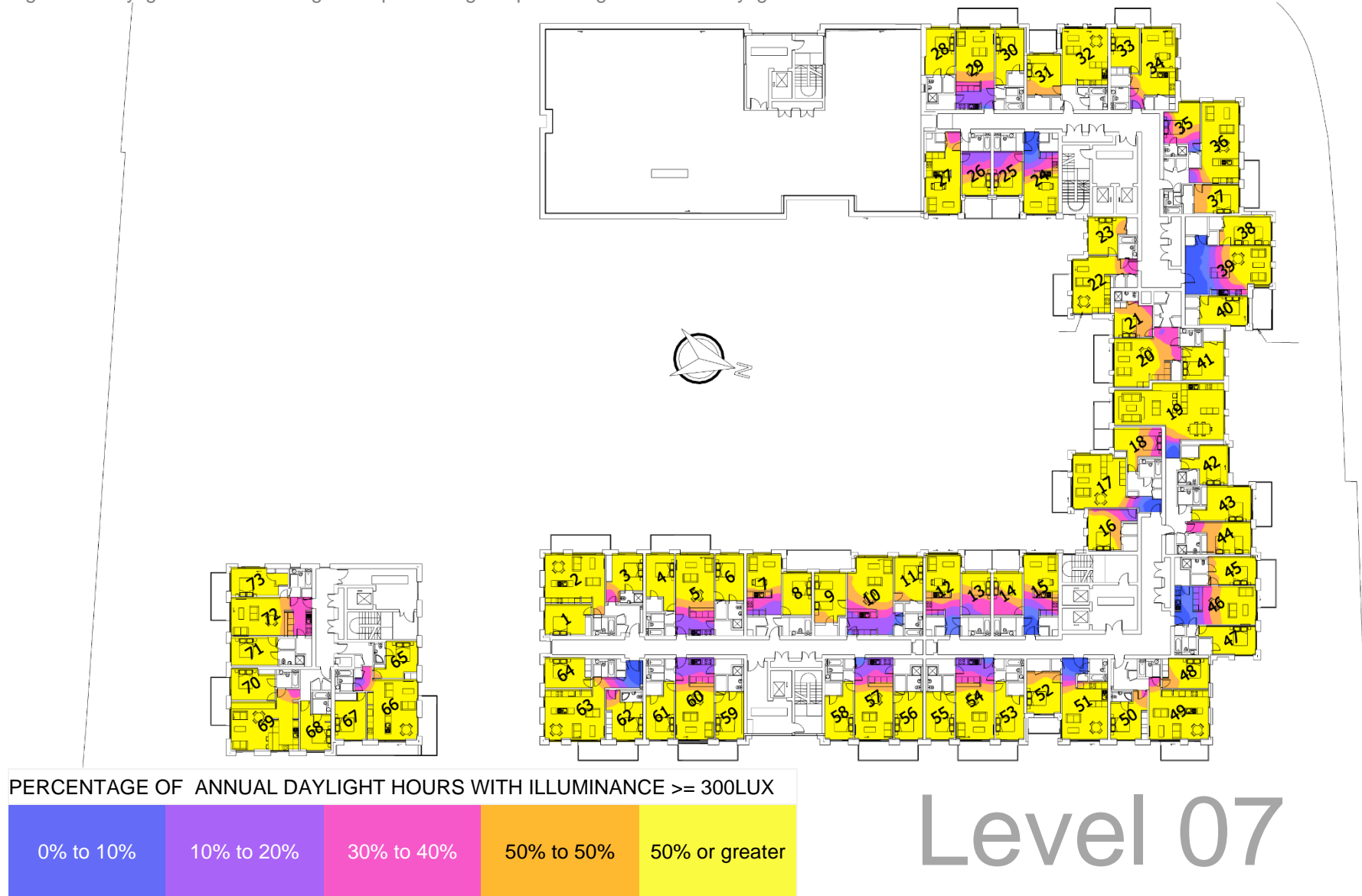
Figure 8 Daylight distribution diagram representing the percentage of annual daylight hours when an illuminance of 300 lux is either met or exceed at Level 07.
