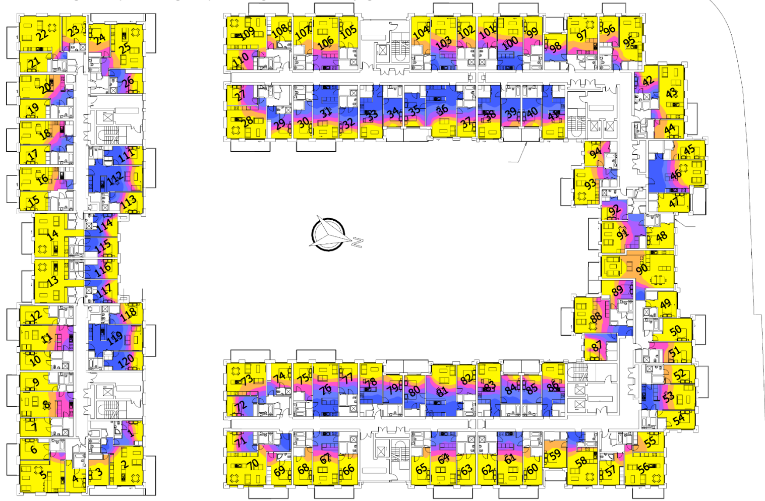
Figure 4 Daylight distribution diagram representing the percentage of annual daylight hours when an illuminance of 300 lux is either met or exceed at Level 03.
