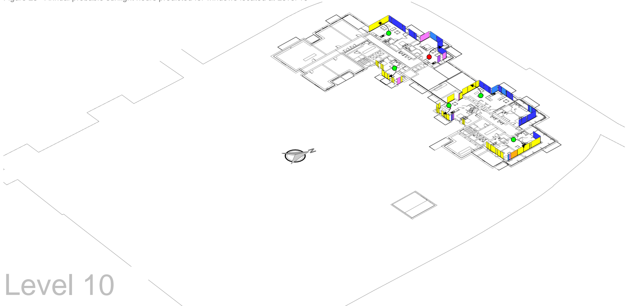
Figure 25 Annual probable sunlight hours predicted for windows located at Level 10
