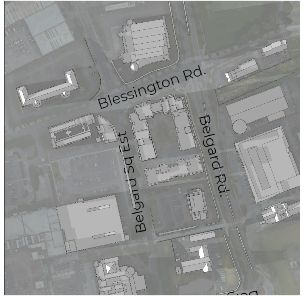
Shadows Cast at 6pm (UTC+0) on the 21 st March - After Development Scenario
