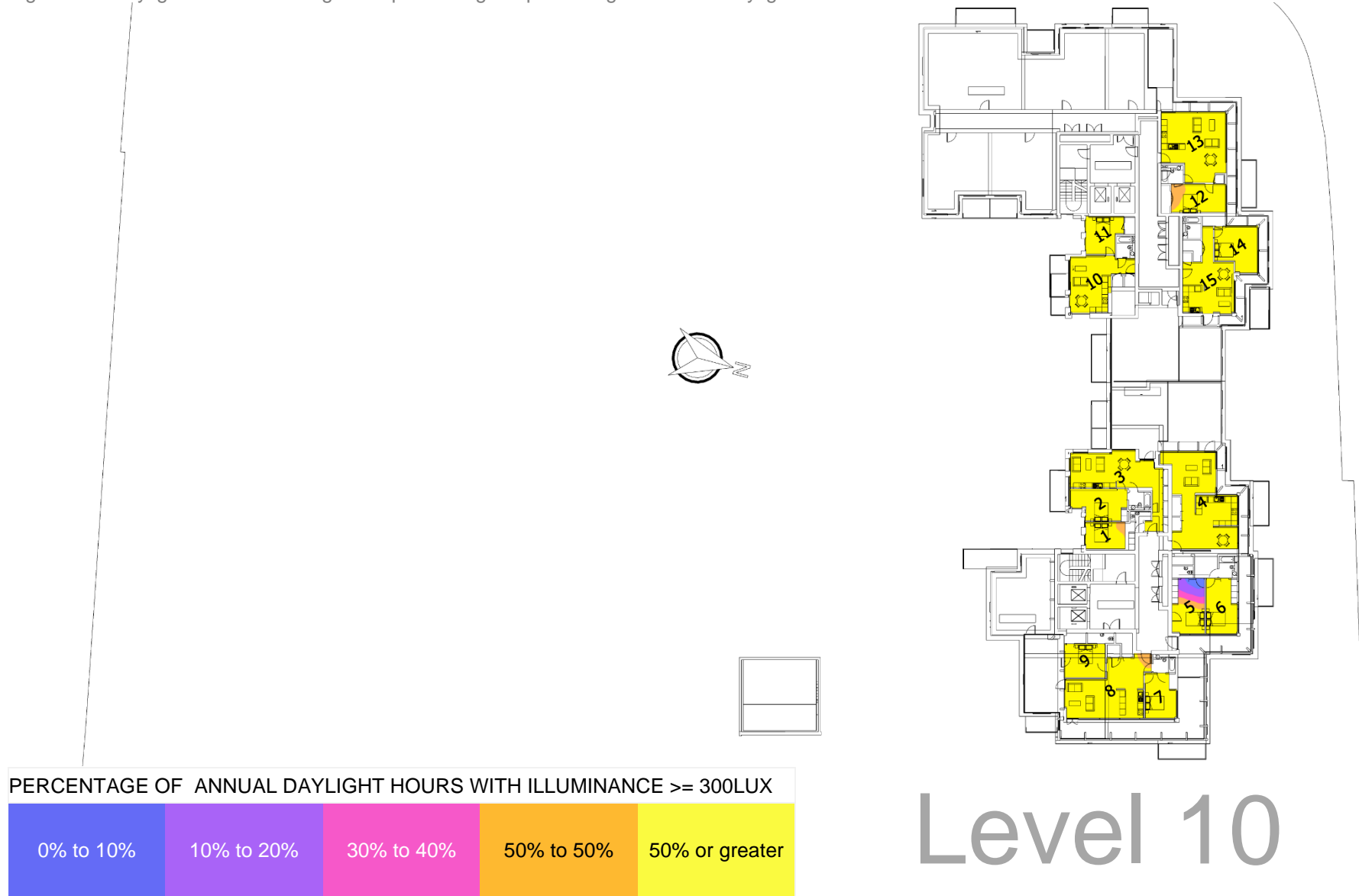
Figure 11 Daylight distribution diagram representing the percentage of annual daylight hours when an illuminance of 300 lux is either met or exceeded at Level 10.
