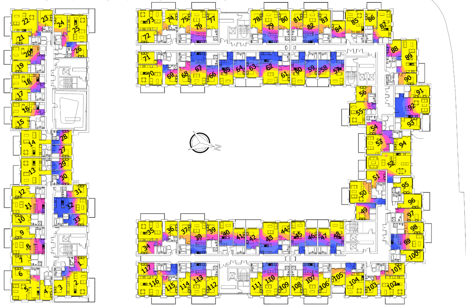
Figure 6 Daylight distribution diagram representing the percentage of annual daylight hours when an illuminance of 300 lux is either met or exceed at Level 05.
