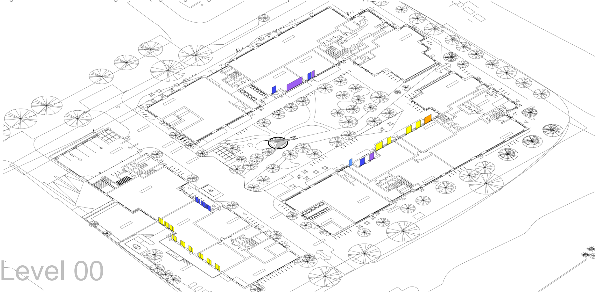
Figure 27 Annual Probable Sunlight Hours (registering during winter months 21 st September to 21 st March) predicted for windows located at Level 00
