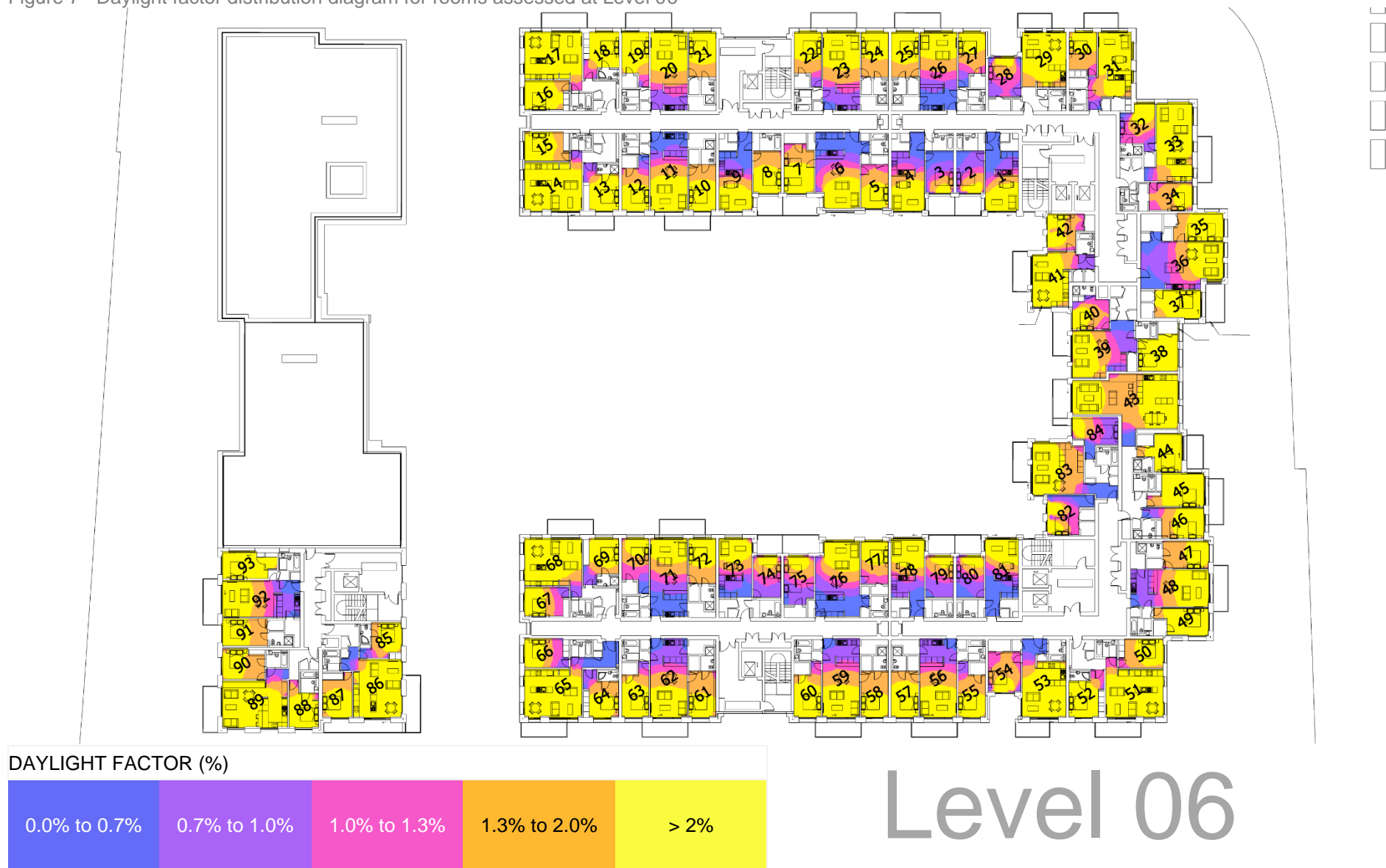
Figure 7 Daylight factor distribution diagram for rooms assessed at Level 06
