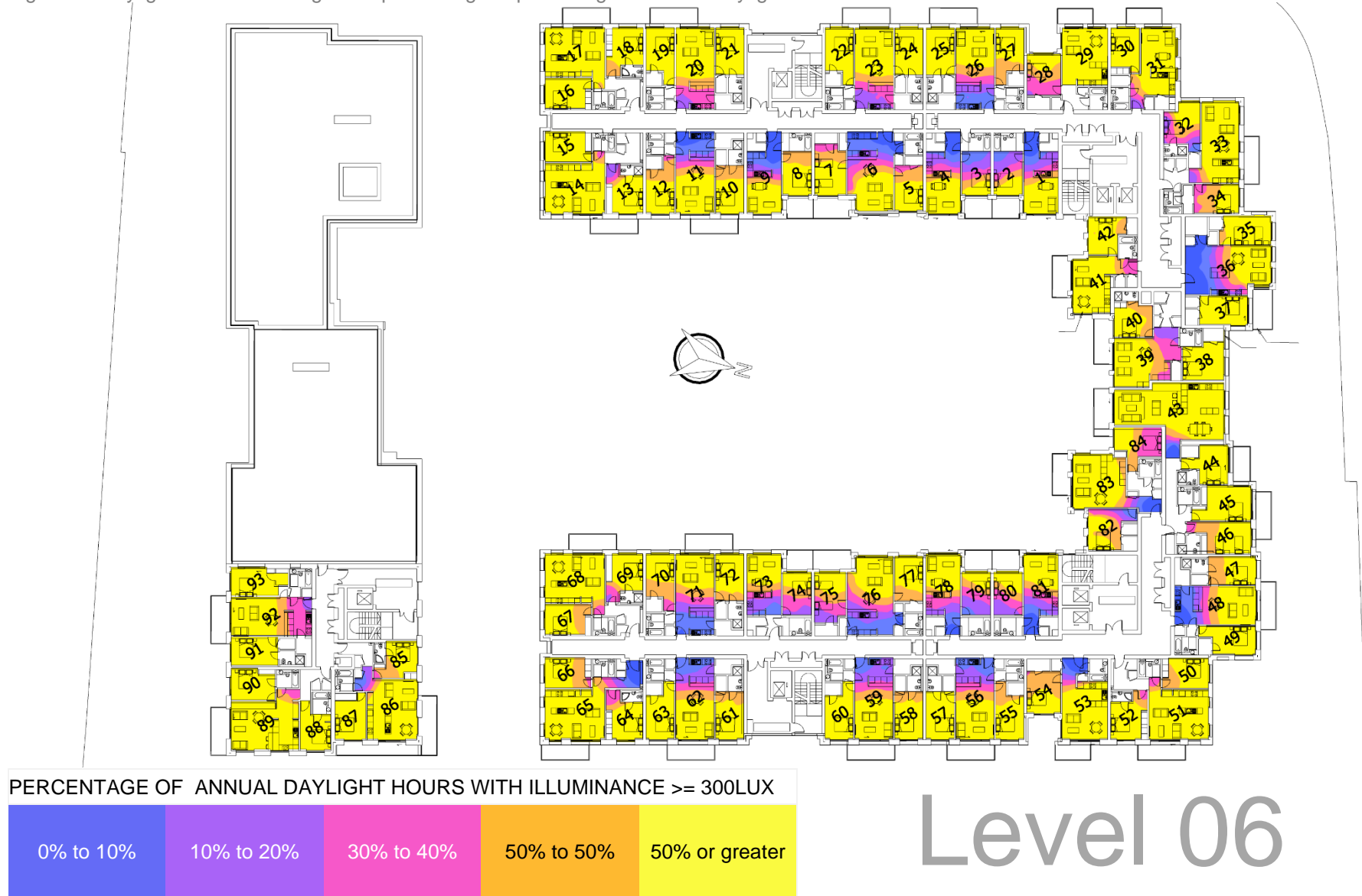
Figure 7 Daylight distribution diagram representing the percentage of annual daylight hours when an illuminance of 300 lux is either met or exceed at Level 06.
