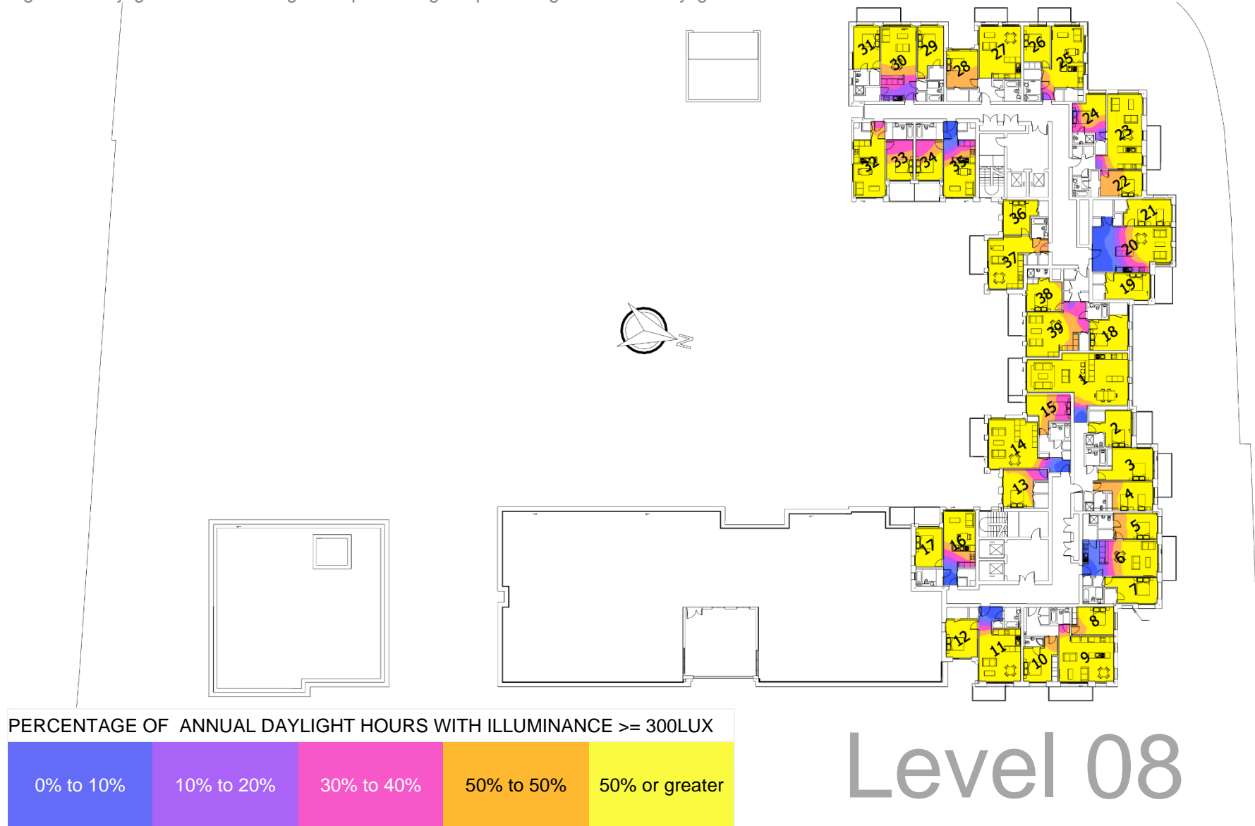
Figure 9 Daylight distribution diagram representing the percentage of annual daylight hours when an illuminance of 300 lux is either met or exceed at Level 08.
