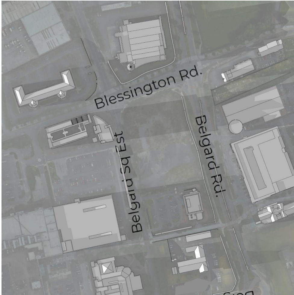
Shadows Cast at 6pm (UTC+0) on the 21 st March - Before Development Scenario
