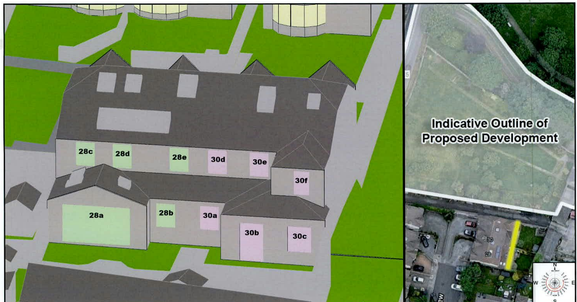
Figure 6.7: Left - Highlighted areas indicate the position of assessed windows., Right - Aerial view of assessed location
