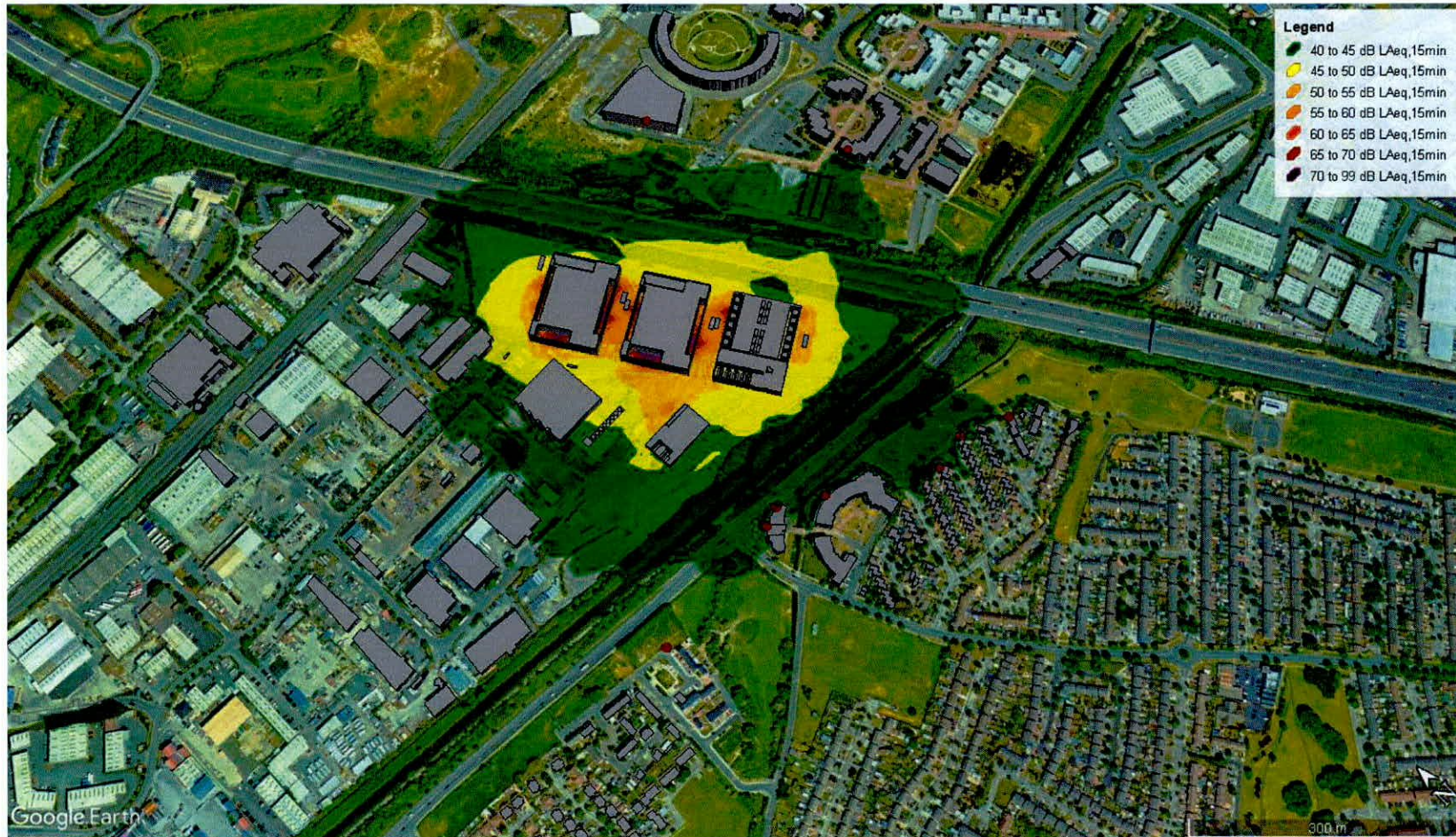
Figure 3 Scenario A – Proposed Data storage facility – Normal Operation (Day/Evening) Noise Contour
