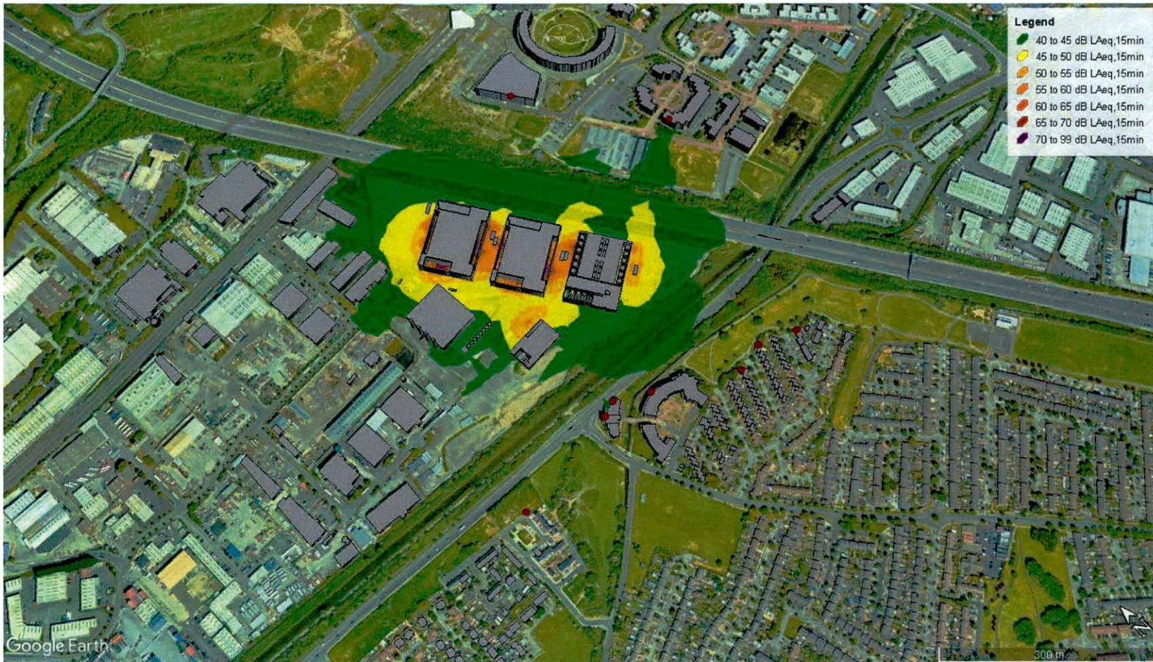
Figure 4 Scenario B – Proposed Data storage facility – Normal Operation (Night) Noise Contour
