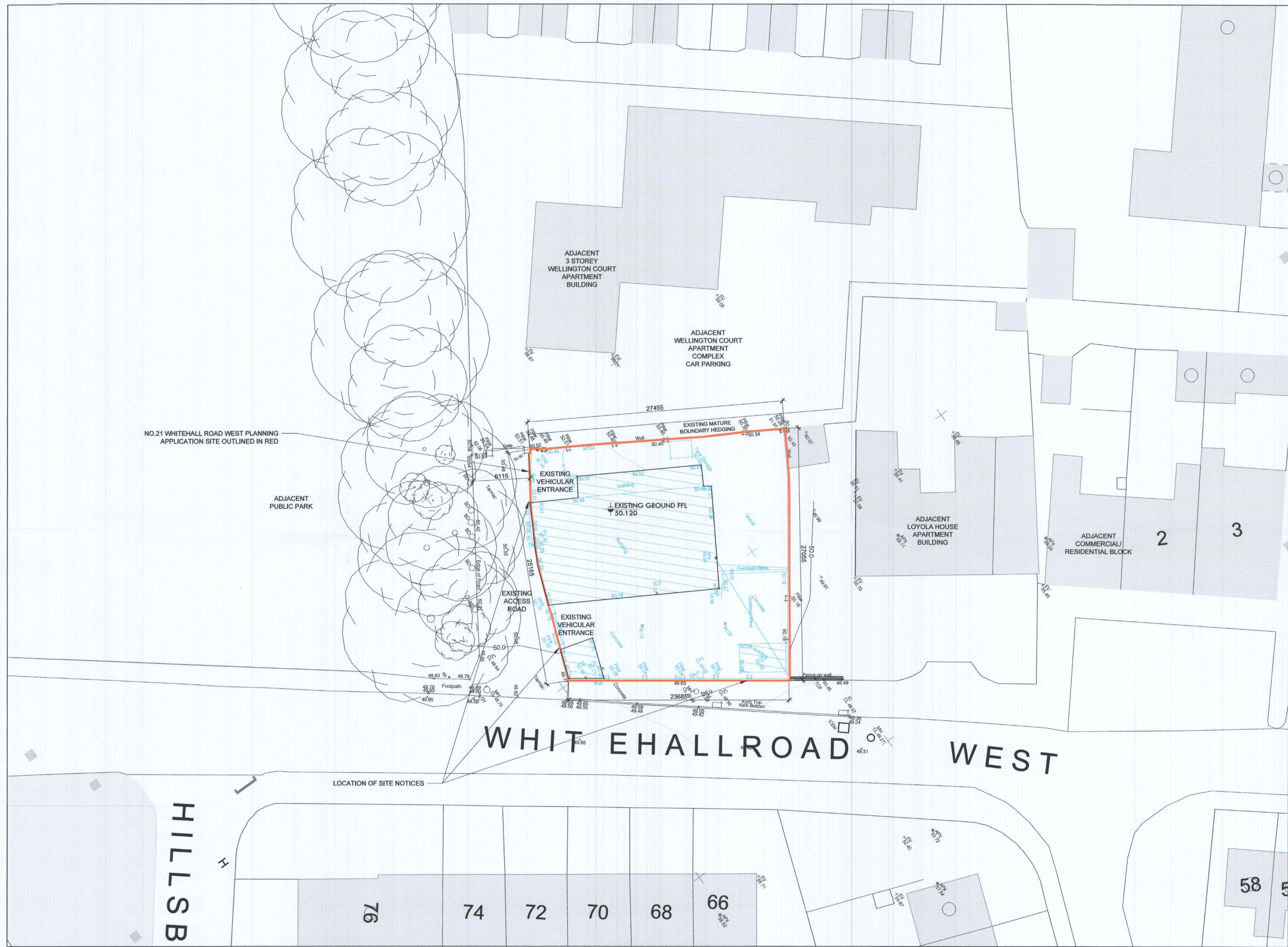
01 EXISTING SITE SURVEY LAYOUT PLAN DEMOLITION SHOWN IN BLUE COLOUR 1:200 @ A1
