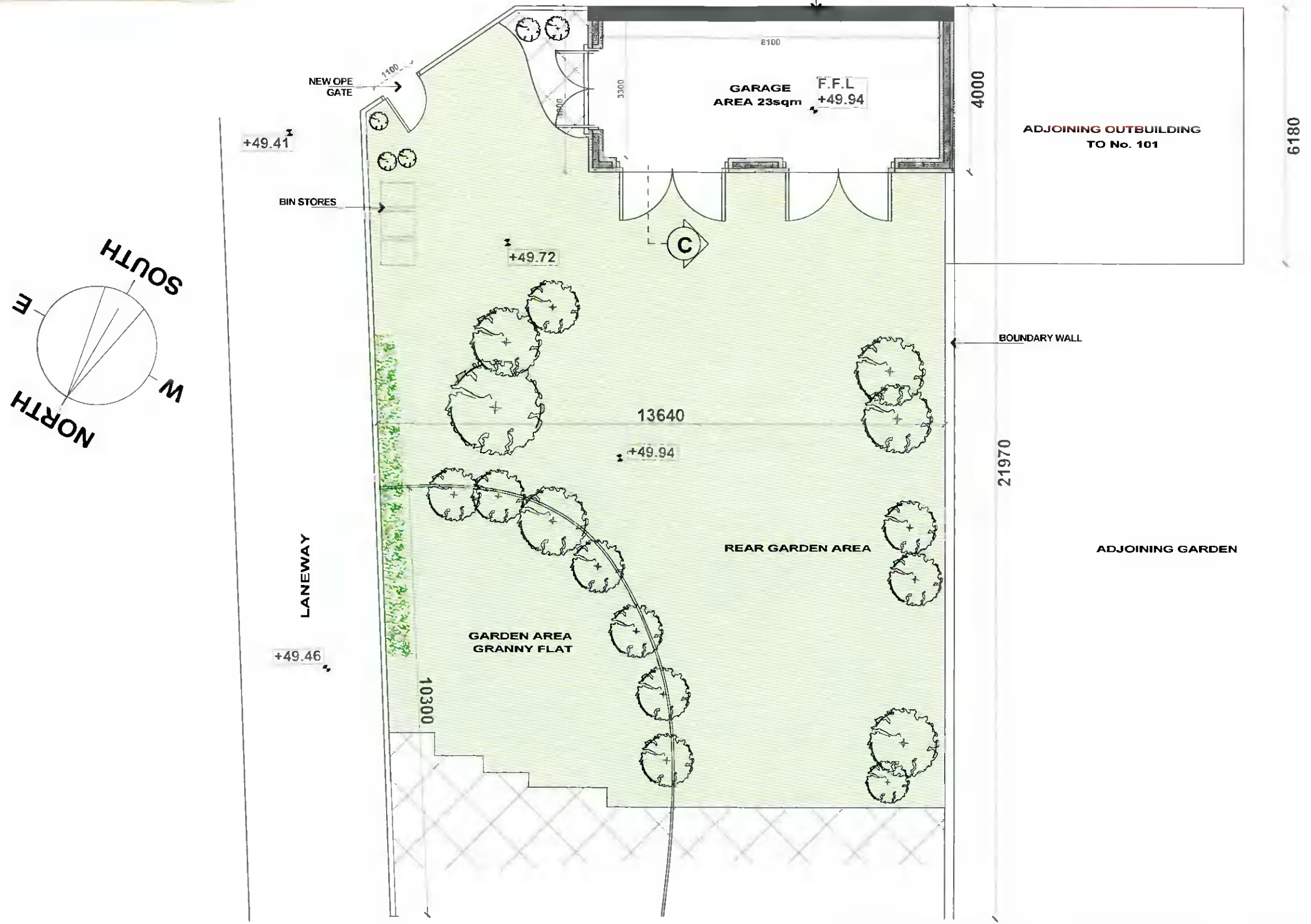
PROPOSED GARAGE PLAN SCALE : 1 / 100 @ A3
