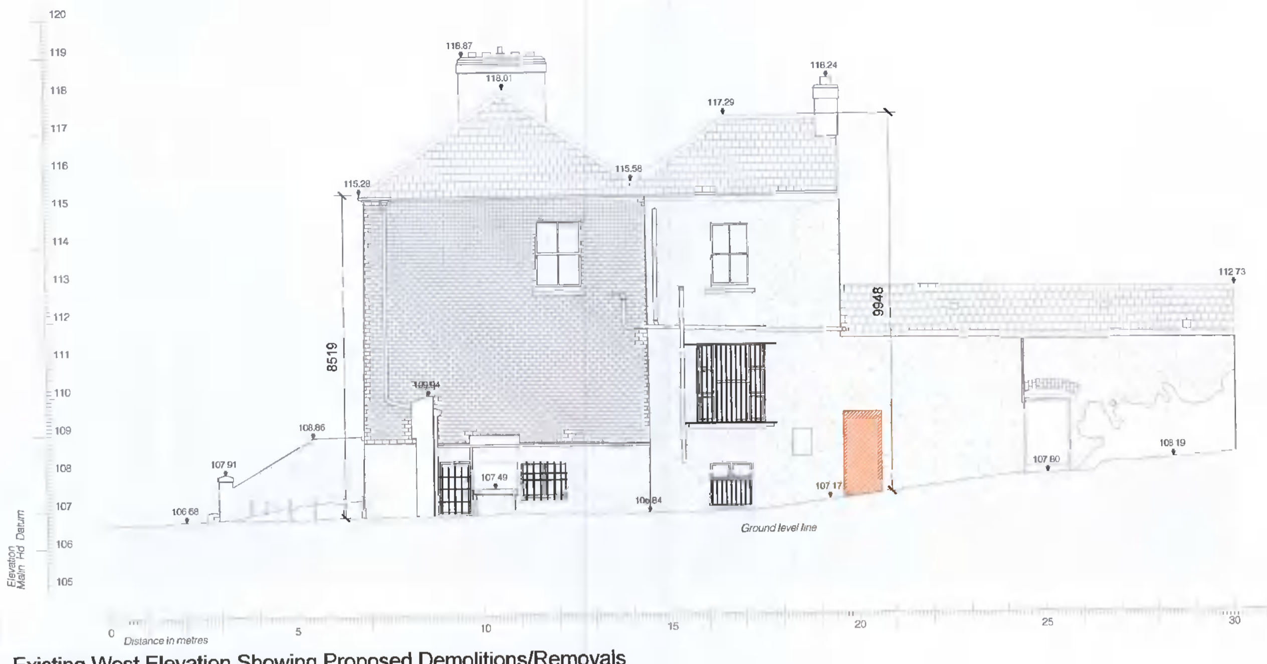
Existing West Elevation Showing Proposed Demolitions/Removals SCALE 1:100
