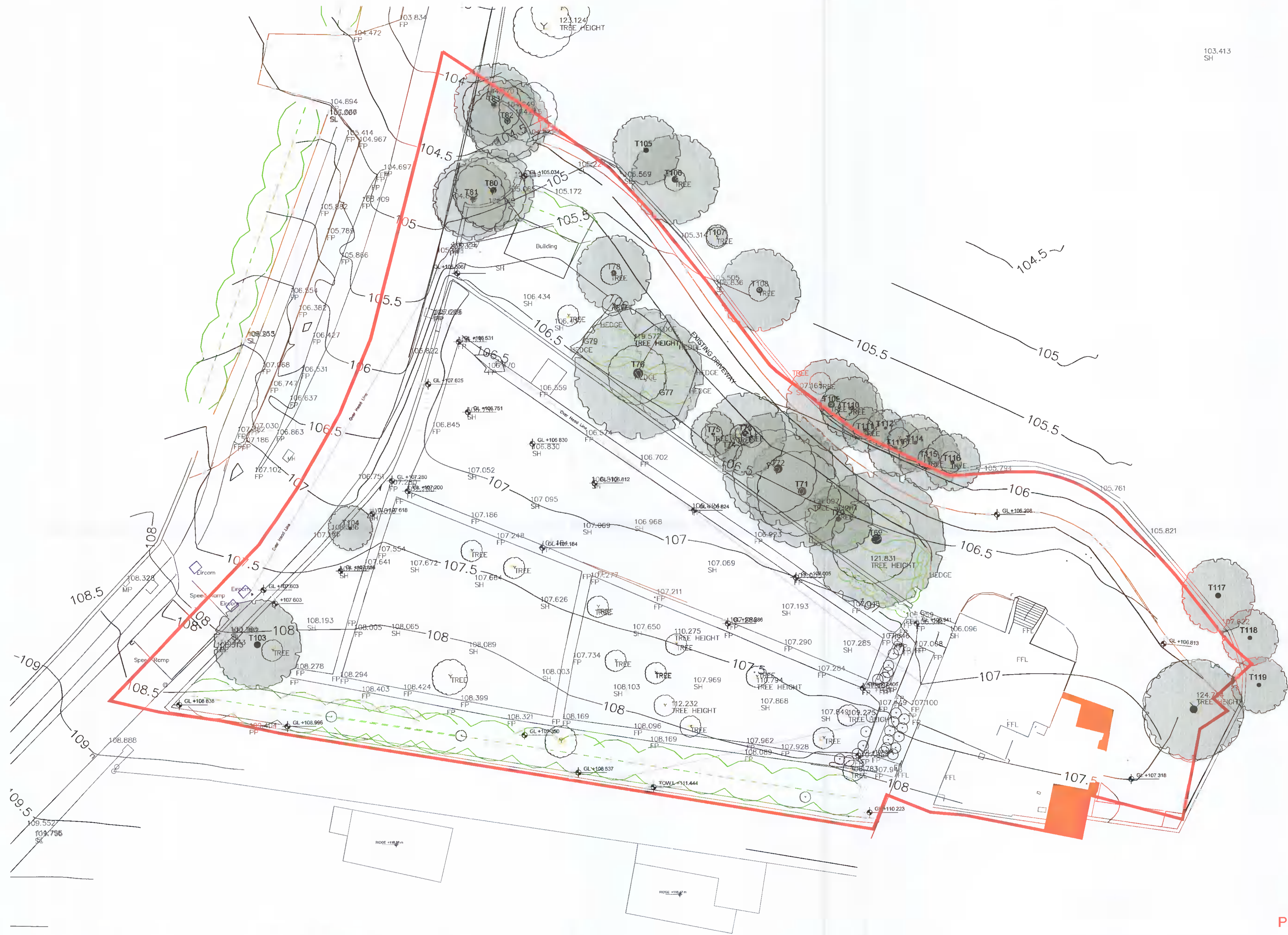
EXISTING SITE LAYOUT PLAN SHOWING STRUCTURES TO BE DEMOLISHED SCALE 1:200
