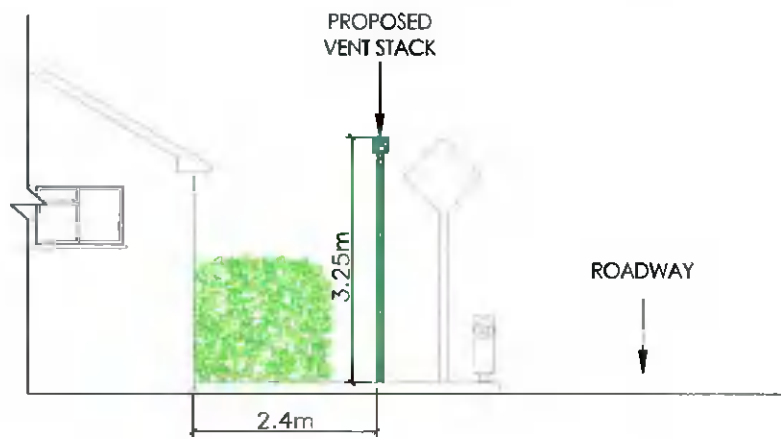
SIDE ELEVATION - WEST FACING: (1:100/A3)
