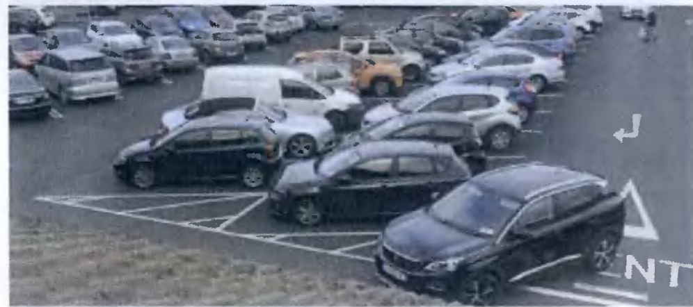
Spaces at angle to assist reduced aisle width show as 90deg spaces on tracking plan.
