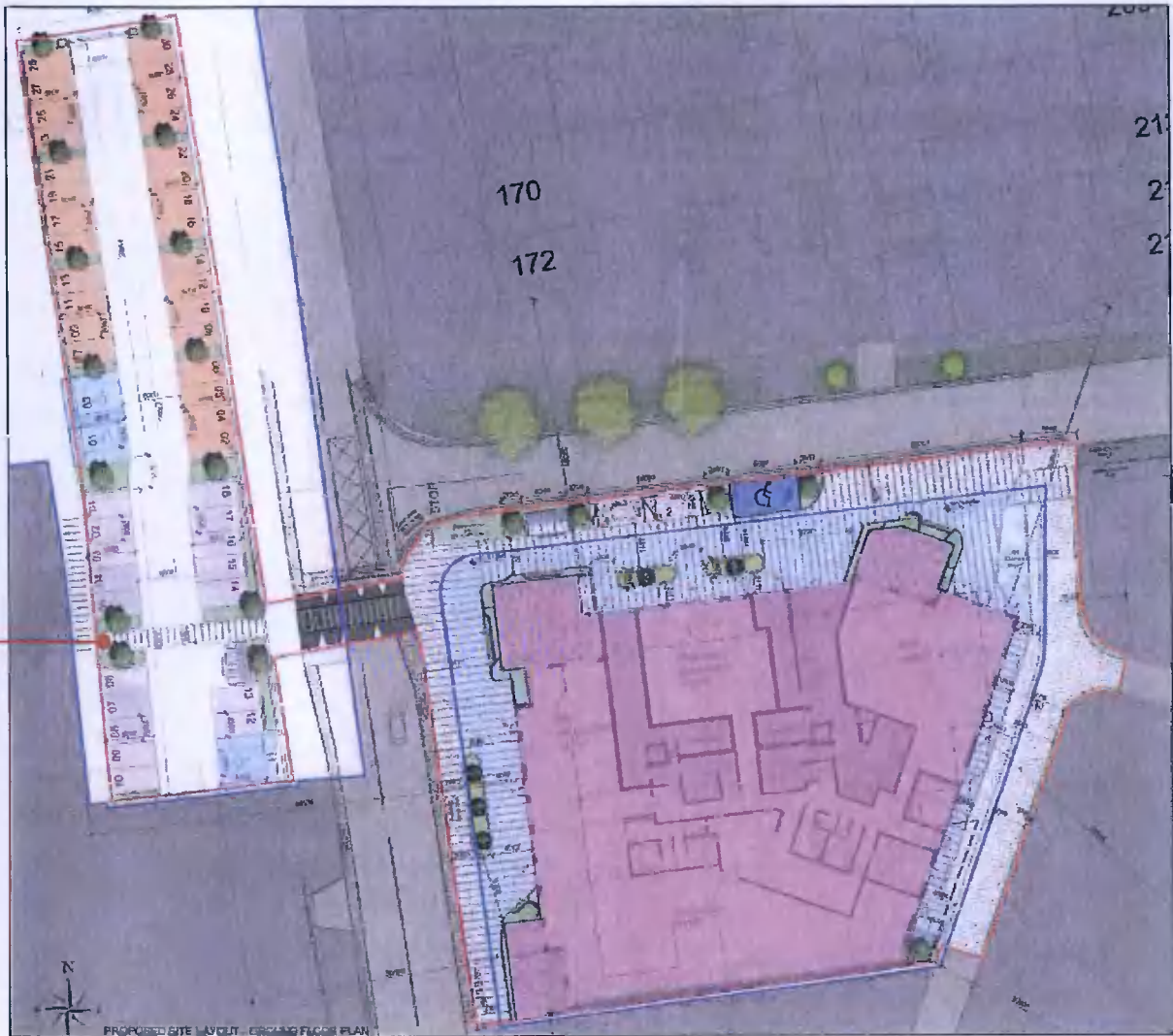
Figure 13.0 Proposed site plan layout provided at further information stage highlighting car parking and foot path provision.
