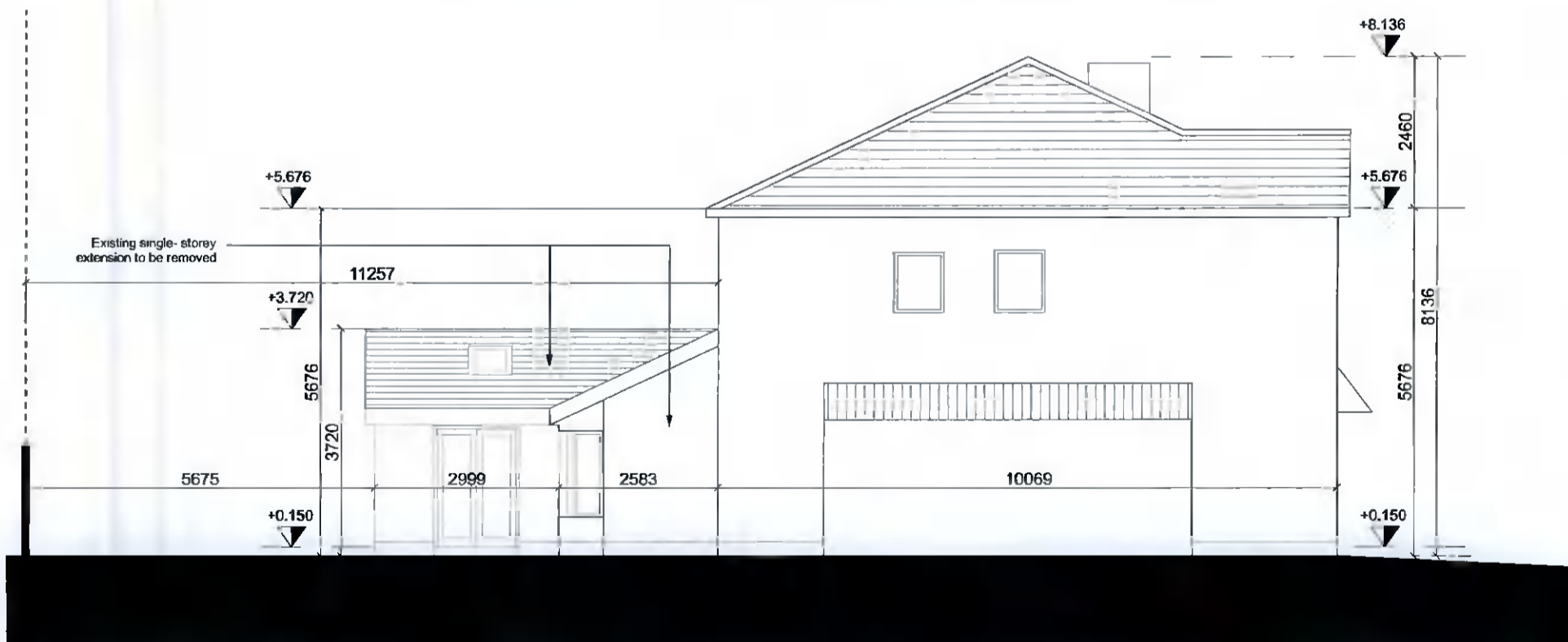
EXISTING SIDE ELEVATION 1:100
