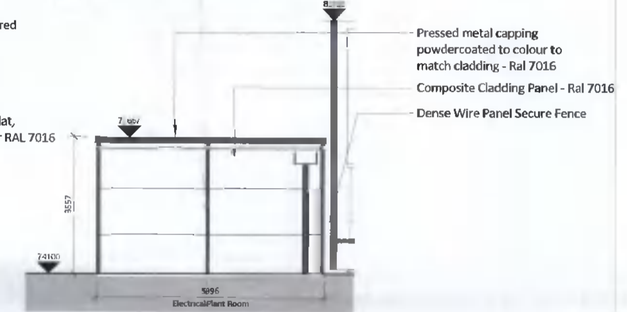
6 Plant Rooms East Elevation 1 : 100
