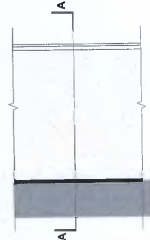
PROPOSED WALL TYPE 02 1800MM HIGH CONCRETE BLOCK WALL, PLASTERED BOTH SIDES, WITH CONCRETE CAPPINGS
